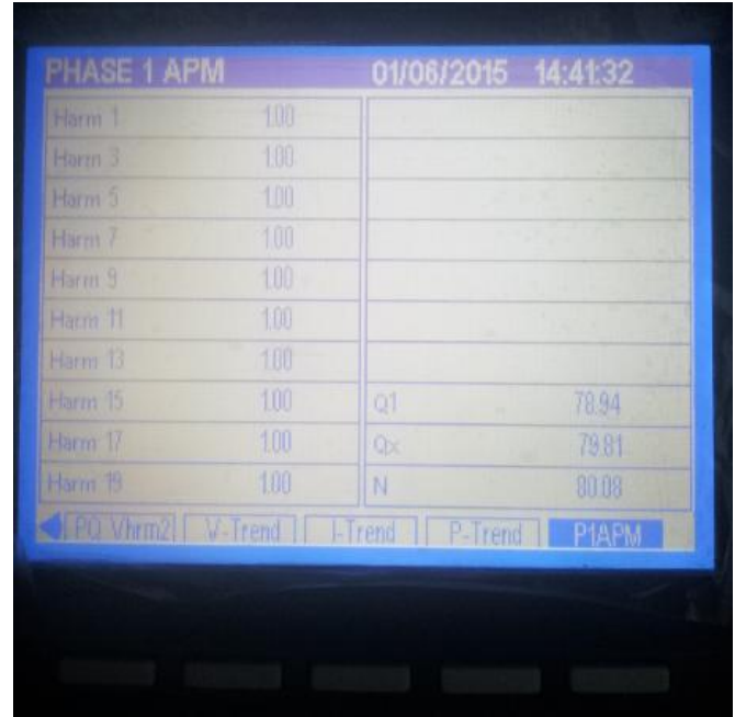
Fig. 3 Harmonic distortion in PCC with only heater connected
