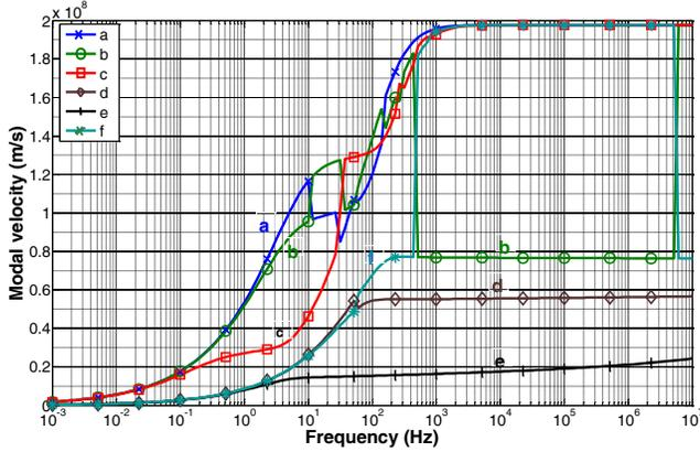
Fig. 1. Modal velocity characteristics of natural modes of propagation for the 110 kV underground cable with mode switching
