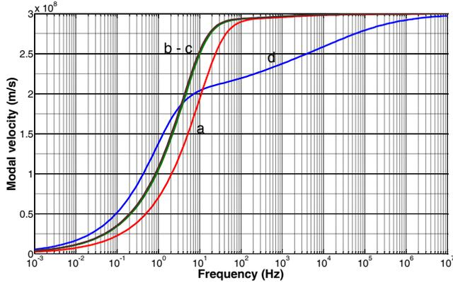
Fig. 8. Modal velocity characteristics of natural modes of propagation for the 110 kV overhead lines without mode switching
