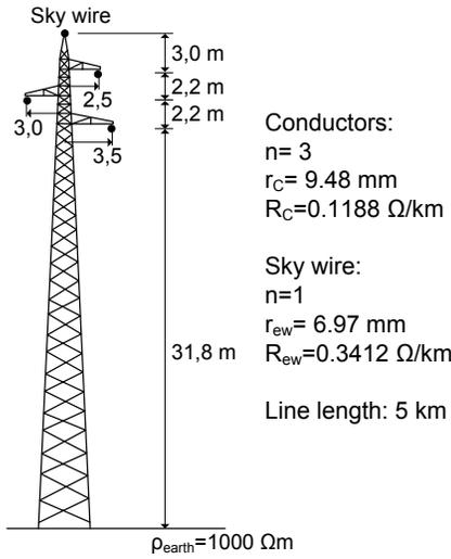
Fig. 7. Data and geometry for 110 kV three phase overhead line
