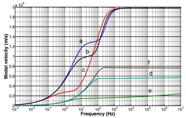
Fig. 3. Modal velocity characteristics of natural modes of propagation for the 110 kV underground cable without mode switching
