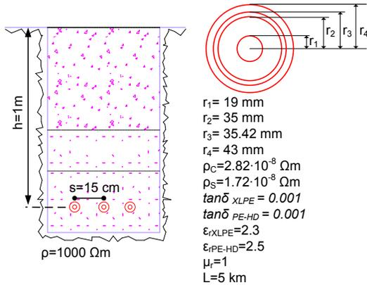
Fig. 2. Data and geometry for 110 kV three phase underground cables
