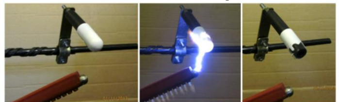
Fig 7: one-time-indicator. Left: initial state. Middle: during lightning impulse. Right: broken bulb, after lightning.
