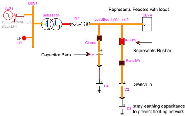
Fig. 12 Equivalent circuit for studying back-to-back switching
