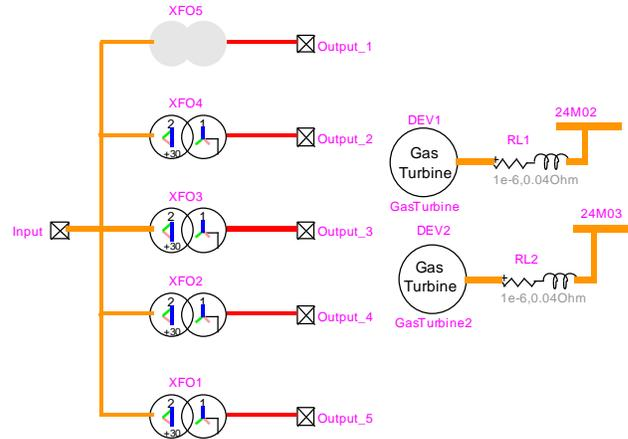
Fig. 3 Substation transformers
