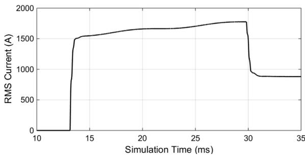
Fig. 7 RMS of maximum inrush current following single bank energization
