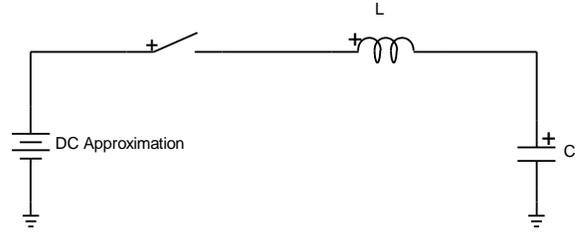
Fig. 5 Simplified circuit to study energization transients
