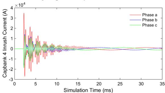
Fig. 10 Max Inrush Current Peak (Switch in 20 Mvars Cap4)
