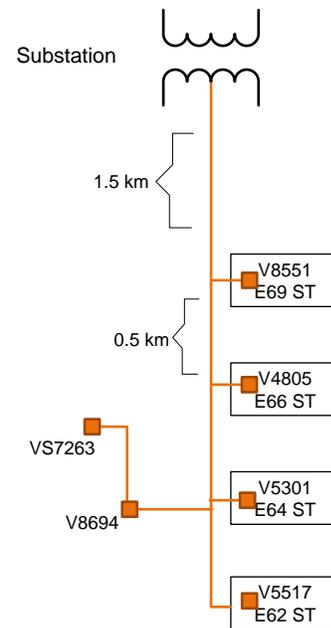
Fig. 8 A feeder with 6 network transformers
