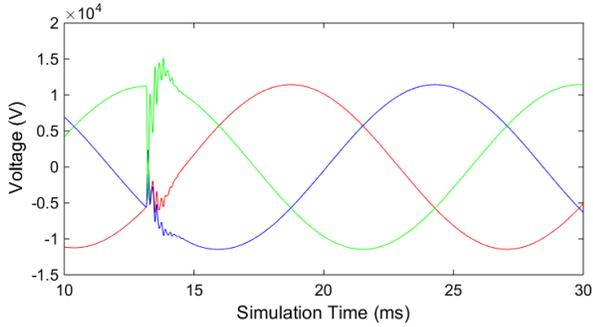
Fig. 9 Overvoltage at the middle of feeder for 100% summer loading
