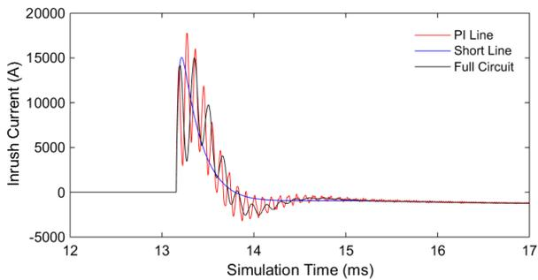
Fig. 13 Max inrush current following single bank energization, with full and equivalent circuits
