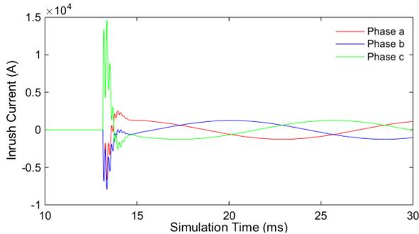
Fig. 6 Maximum inrush current following single bank energization
