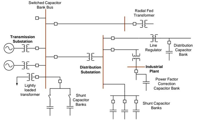
Fig. 4 Capacitors in Power Systems
