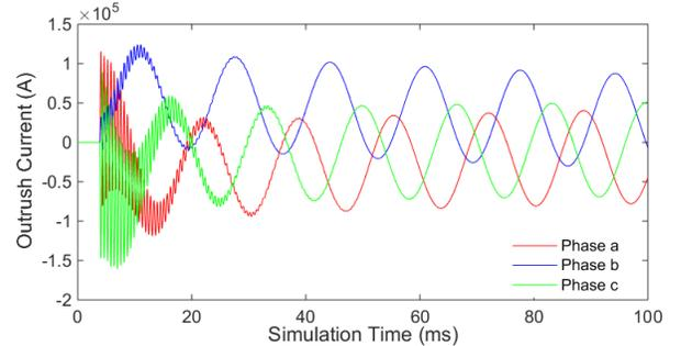
Fig. 11 Typical short circuit currents when capacitors are in service
