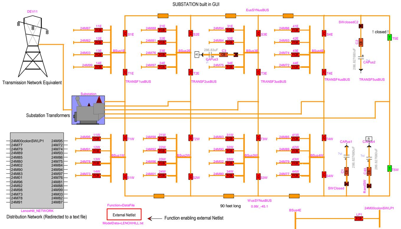
Fig. 1 Substation design: circuit breakers, feeder starts, capacitor banks and busbars
