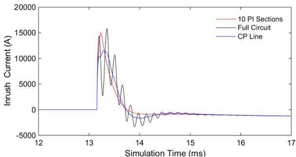
Fig. 14 Max inrush current following single bank energization, with full and equivalent circuits
