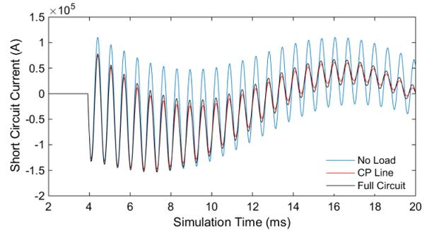
Fig. 16 Short circuit currents on phase c when capacitors are in service
