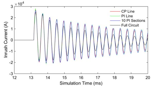
Fig. 15 Max inrush current when one bank is in service, with full and equivalent circuits
