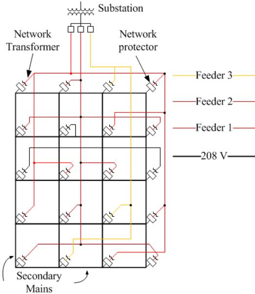
Fig. 2 Simplified topology of a grid network
