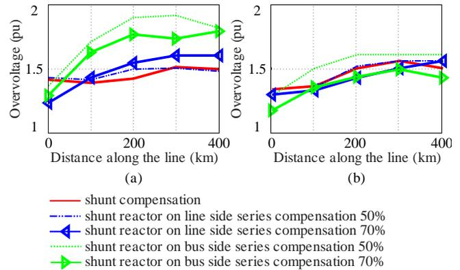
Fig. 12. Overvoltages along the line with reactive compensation on receiving terminal: (a) 50% shunt compensation; (b) 70% shunt compensation.
