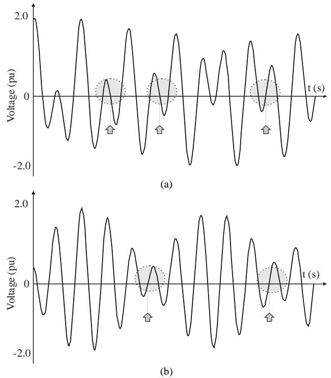
Fig. 3. Voltage across the circuit breaker poles for: (a) high shunt compensation degree; (b) low shunt compensation degree.
