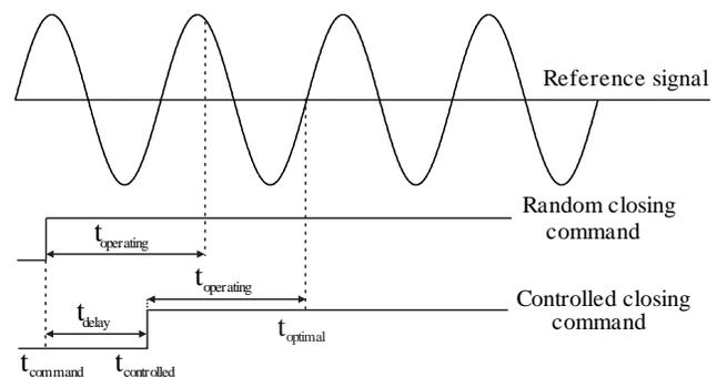
Fig. 1. Controlled switching scheme.
