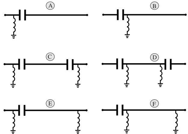
Fig. 5. Schemes of series and shunt compensated lines.
