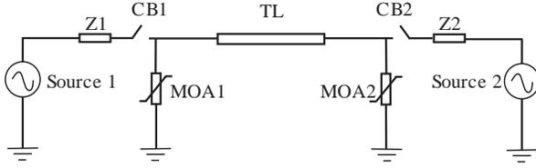
Fig. 6. Scheme of power system used in the cases studies.
