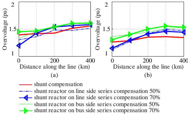
Fig. 18. Overvoltages along the line with reactive compensation on receiving terminal: (a) 50% shunt compensation; (b) 70% shunt compensation.
