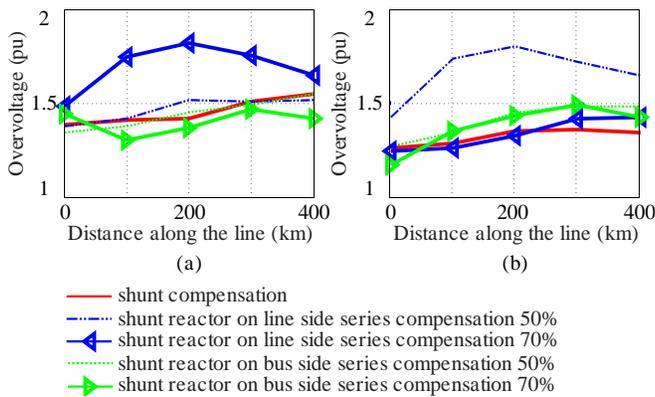
Fig. 14. Overvoltages along the line with reactive compensation at both line ends: (a) 50% shunt compensation; (b) 70% shunt compensation.
