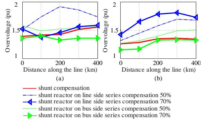
Fig. 16. Overvoltages along the line with series compensation at line sending terminal, and shunt compensation at both line terminals: (a) 50% shunt compensation; (b) 70% shunt compensation.
