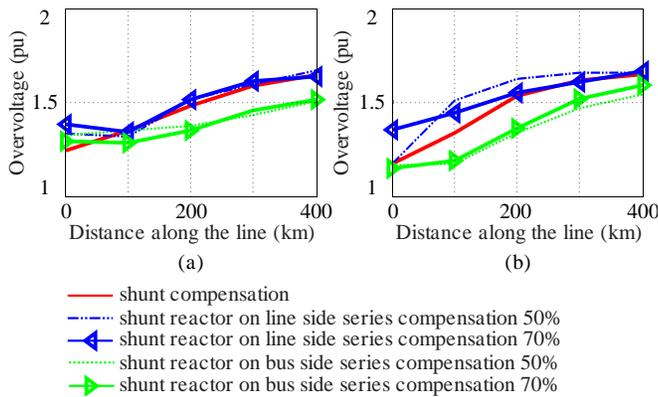
Fig. 10. Overvoltages along the line: (a) 50% shunt compensation; (b) 70% shunt compensation.
