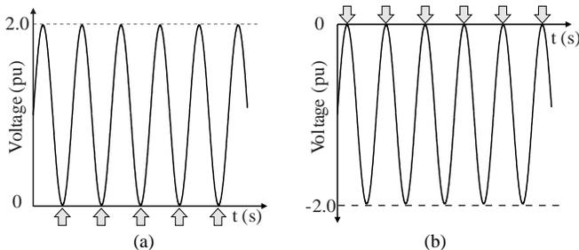
Fig. 2. Voltage across the circuit breaker poles for shunt reactor compensated line with trapped charge with: (a) negative polarity; (b) positive polarity.
