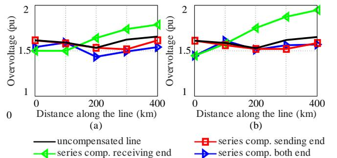
Fig. 9. Overvoltages along the purely series compensated line with: (a) 50% series compensation; (b) 70% series compensation.
