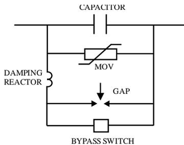
Fig. 4. Typical circuit of series capacitor bank.
