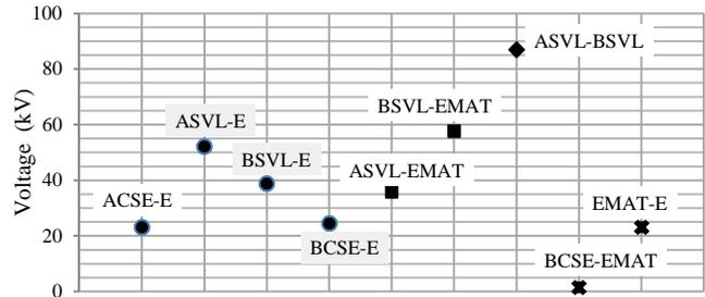
Fig. 15. Voltage of sheath and earth mat with 1  $\mu$ H in SUBA side SVL connection.
