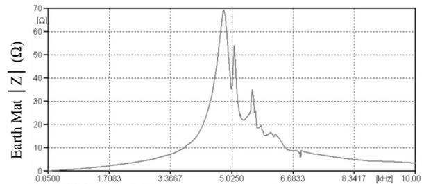
Fig. 9. Frequency scan looking into SUBX earth mat with cables and all earth wires connected.
