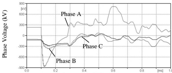
Fig. 10. Conductor voltages at CSE.
