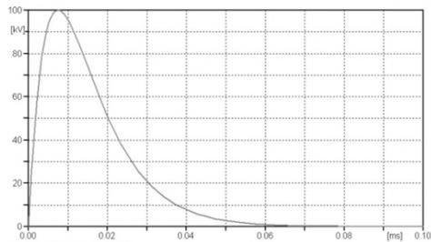
Fig. 6. An 8/20  $\mu\text{s}$  impulse applied to an isolated cable.
