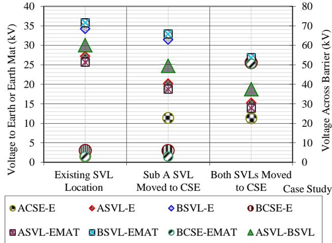
Fig. 18. Sheath voltages for different SVL and earthing arrangements with earth mat as pure resistance and perfect connections.
