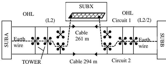
Fig. 2. Circuit diagram.
