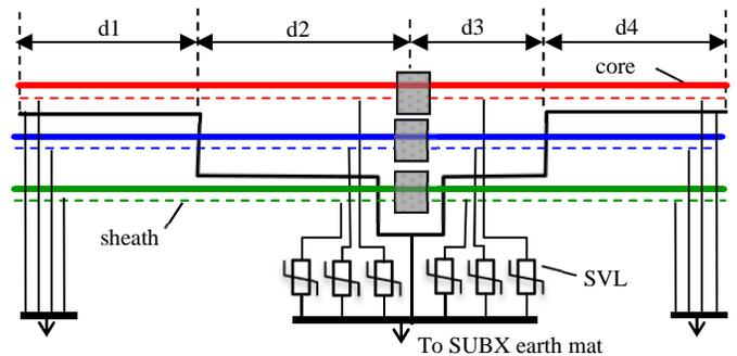
Fig. 3. Cable junction box arrangement.
