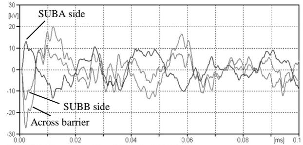
Fig. 7. Sheath voltage to true earth and across insulation barrier for symmetric connection.
