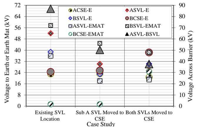
Fig. 16. Sheath voltages for different SVL and earthing arrangements.
