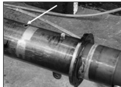
Fig. 1. Damaged cable joint.
