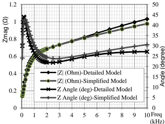
Fig. 12. Earth mat impedance for detailed and approximate models.
