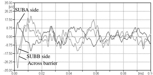
Fig. 8. Sheath voltage to true earth and across insulation barrier for asymmetric connection.
