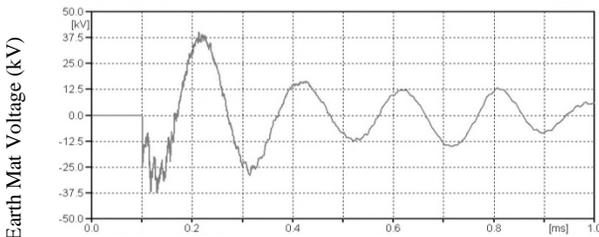
Fig. 11. Earth mat voltage for lumped model.
