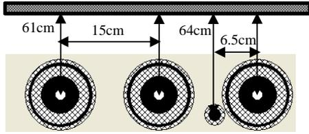
Fig. A.2. Cable layout, spacing and trench depth.
