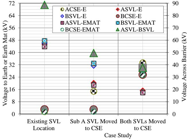
Fig. 17. Sheath voltages for different SVL and earthing arrangements with earth mat as pure resistance.
