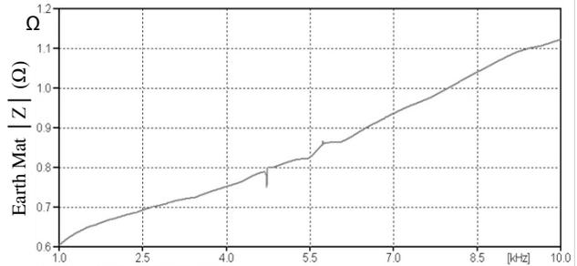
Fig. 13. Frequency scan of the SUBX earth mat approximate model with cables and all earth wires connected.
