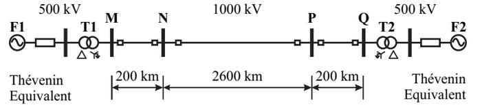
Fig. 3. Simulated power system single-line diagram.
