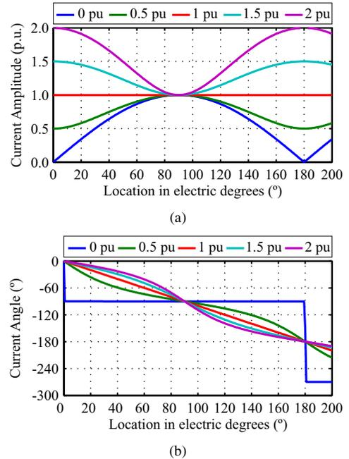
Fig. 2. Current phasor profiles along a  $\lambda/2^+$  for different load flow conditions: (a) amplitude and (b) angle.
