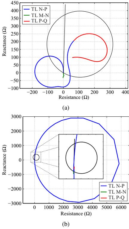
Fig. 5. Apparent impedance calculated by the relay unit  $Z_{AG}$  for simulated (a) AG and (b) ABC faults along the system lines.
