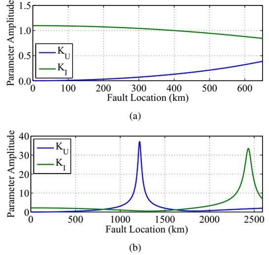
Fig. 7.  $K_U$  and  $K_I$  for fault along a (a) 650 km length line and a (b) 2 600 km length line.
