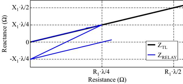
Fig. 10.  $\lambda/2^+$  positive sequence impedance and apparent impedance calculated by a  $Z_{AG}$  unconventional distance relay unit at Bus N from internal faults considering  $k_1$  and  $k_2$  calculated for the exact fault location (Case 2).
