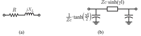
Fig. 6. (a) Short line model: used as premise for conventional distance protection; (b) Long line model: used as premise for unconventional distance protection.
