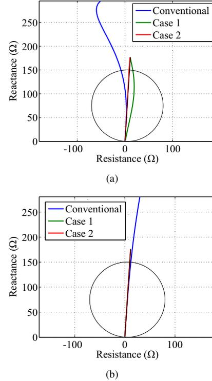
Fig. 8. Apparent impedances calculated by a  $Z_{AG}$  relay unit at a 800 km 500 kV transmission line for (a) AG and (b) ABC faults along its extension considering 3 formulations: conventional; unconventional with  $k_1$  and  $k_2$  calculated for a fault at the end of transmission line (Case 1) and; unconventional with  $k_1$  and  $k_2$  calculated for the exact fault location (Case 2).
