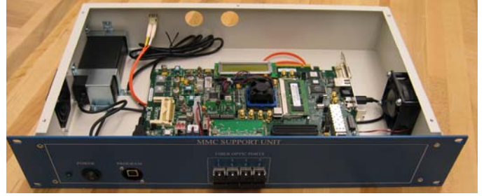
Figure 6. FPGA-based MMC Support Unit
