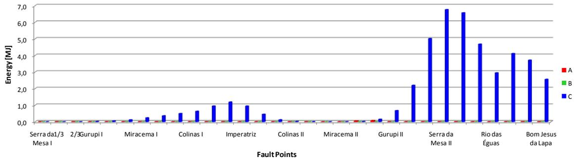
Fig. 15. Energy absorption [MJ] of the surge arresters in Rio das Éguas considering faults along the line.
