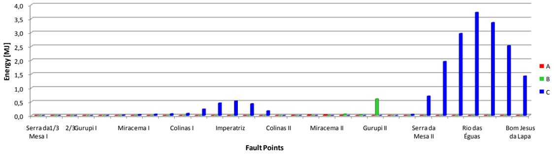
Fig. 14. Energy absorption [MJ] of the surge arresters in Colinas I considering faults along the line.
