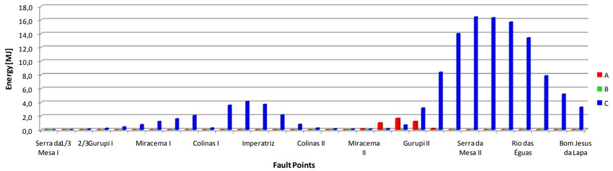
Fig. 16. Energy absorption [MJ] of the surge arresters in Bom Jesus da Lapa considering faults along the line.
