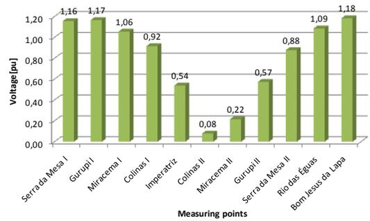
Fig. 4. Steady state voltage profile along the line after energization without fault.
