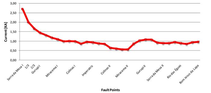
Fig. 12. Maximum currents in the transformer neutral for faults along the line.
