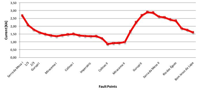
Fig. 11. Maximum fault currents along the AC-Link.
