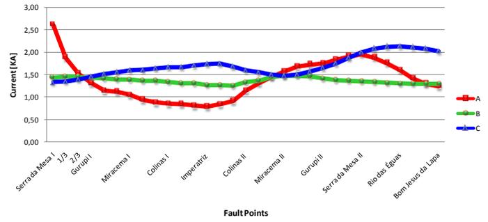
Fig. 10. Maximum currents in the circuit breaker due to A-G Fault along the line.
