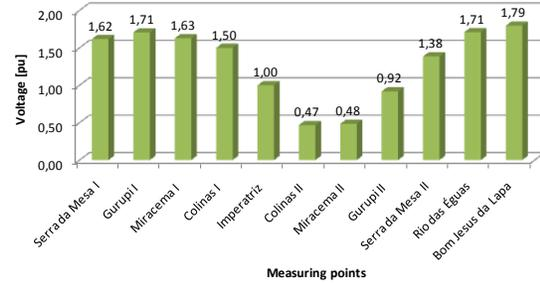
Fig. 3. Maximum transient overvoltages along the line.
