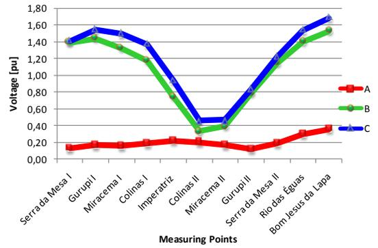
Fig. 7. Maximum transient overvoltage due to A-G Fault at the sending end
