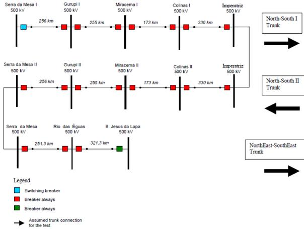
Fig. 1. Single-phase diagram of AC-Link Test – 500 kV.
