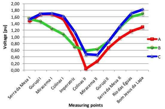
Fig. 8. Maximum transient overvoltage due to A-G Fault in Colinas II.
