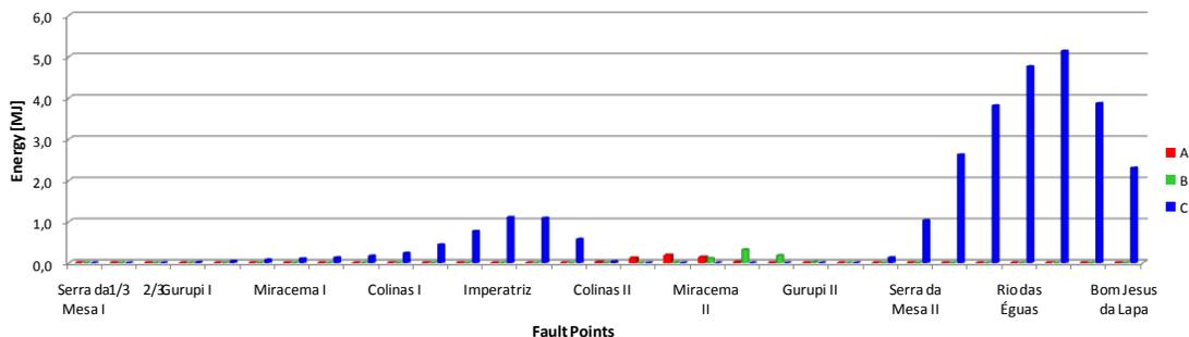
Fig. 13. Energy absorption [MJ] of the surge arresters in Miracema I considering faults along the line.
