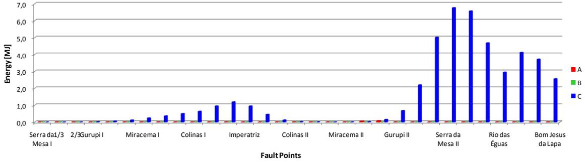
Fig. 15. Energy absorption [MJ] of the surge arresters in Rio das Éguas considering faults along the line.
