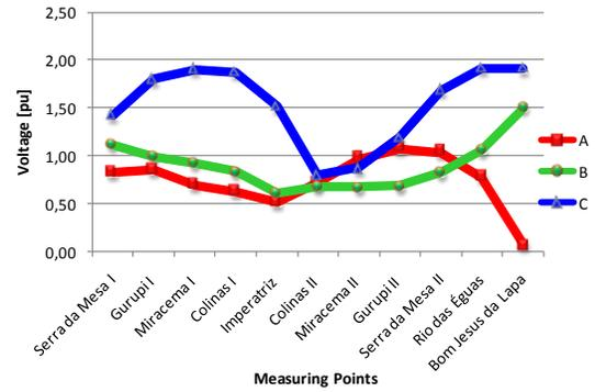
Fig. 9. Maximum transient overvoltage due to A-G Fault at the receiving end
