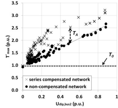
Fig. 11. The highest peak torsional stresses  $T'_{max}$  detected in Case II
