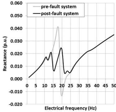
Fig. 4. Reactance curve for pre-fault and post-fault system conditions corresponding to an arbitrary fault and operating conditions of the system
