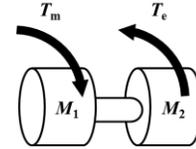
Fig. 3. Applied mechanical system configuration
