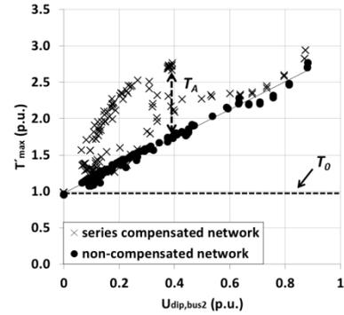
Fig. 10. The highest peak torsional stresses  $T'_{max}$  detected in Case I
