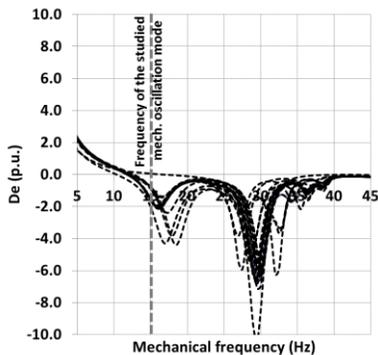
Fig. 8. Subsynchronous damping of the system after the fault clearance in Case II
