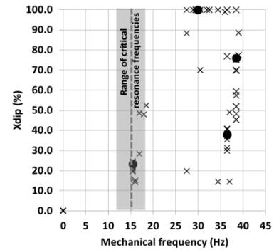
Fig. 6. Reactance dips for pre-fault and post-fault system conditions detected for Case II
