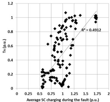
Fig. 12. Average series capacitor (SC) charging during the fault period vs. amplification of torsional stresses in Case I
