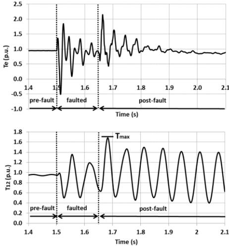
Fig. 9. Electrical torque and torque between masses of the two-mass shaft model for the case of a 150 ms fault at line between bus 4 and SC9
