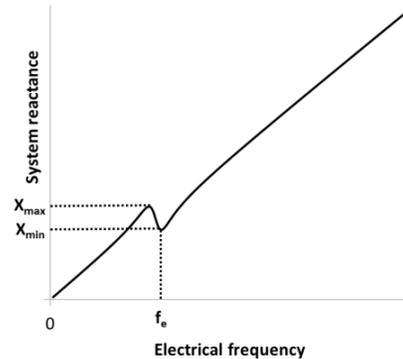
Fig. 1. Detection of the electrical system resonance frequencies
