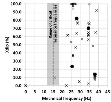
Fig. 5. Reactance dips for pre-fault and post-fault system conditions detected for Case I
