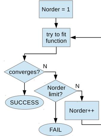
Figure 6: Algorithm for testing minimum order required to converge within desired error
