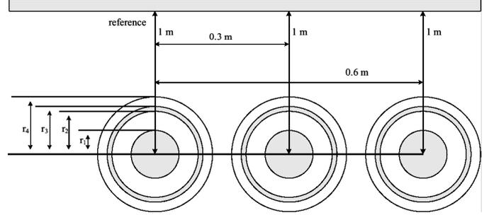
Figure 3: Configuration of underground power cables studied
