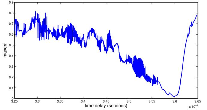
Figure 2: Typical example of VF  $maxerr$  with respect to choice of time delay,  $\tau_m$
