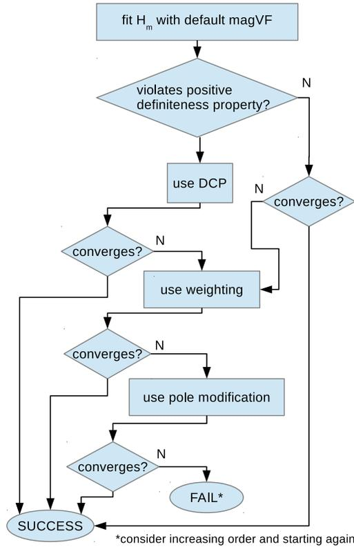
Figure 4: Testing algorithm used to determine effect of magVF modifications with fixed order
