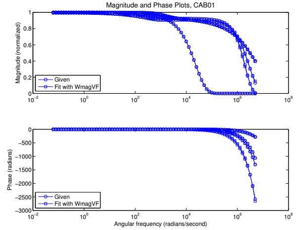
Figure 5: Magnitude and phase plots of all 6 modal propagation functions using 12 poles to fit ( $Norder = 12$ ). Given modal data is superimposed with WmagVF approximation (see Table I for errors)
