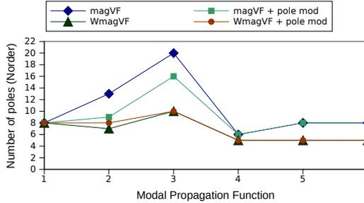
(b) Using magVF/WmagVF, with/without pole modification.
