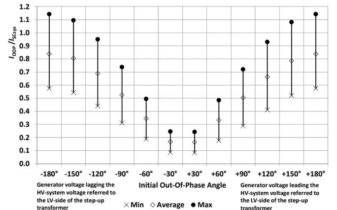
Fig. 10. Ratio of the a.c. component of the out-of-phase breaking current to the a.c. component of the system-source short-circuit breaking current as a function of initial out-of-phase angle
