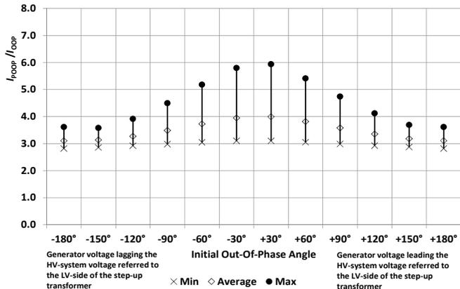
Fig. 13. Ratio of the peak value of the out-of-phase fault current to the out-of-phase breaking current as a function of initial out-of-phase angle
