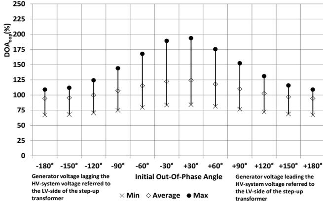
Fig. 11. Degree of asymmetry of the out-of-phase breaking current as a function of initial out-of-phase angle
