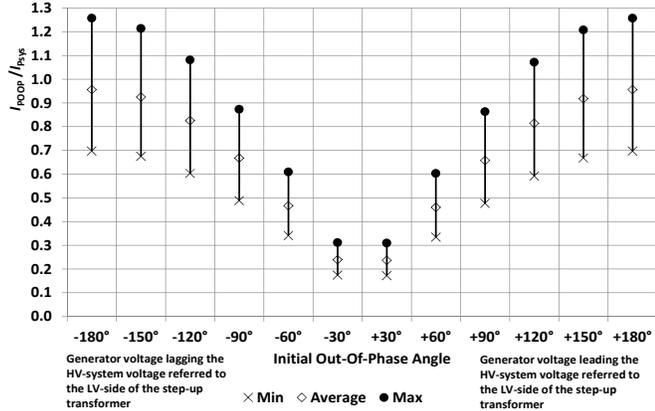
Fig. 12. Ratio of the peak value of the out-of-phase fault current to the peak value of the system-source short-circuit current as a function of initial out-of-phase angle
