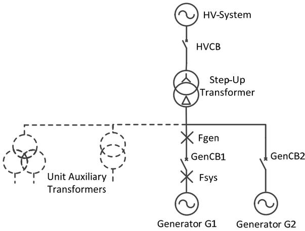
Fig. 3. Power station layout with two generators connected to a two-winding step-up transformer
