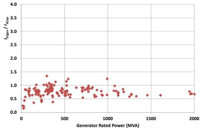
Fig. 7. Ratio of the a.c. component of the generator-source short-circuit breaking current to the a.c. component of the system-source short-circuit breaking current as a function of generator rated power
