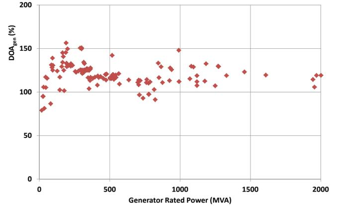
Fig. 8. Degree of asymmetry of the generator-source short-circuit breaking current as a function of generator rated power
