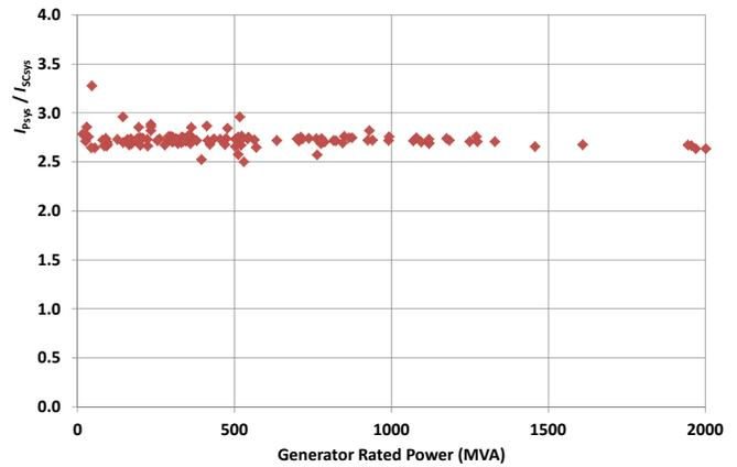
Fig. 6. Ratio of the peak value of the system-source short-circuit current to the system-source short-circuit breaking current as a function of generator rated power
