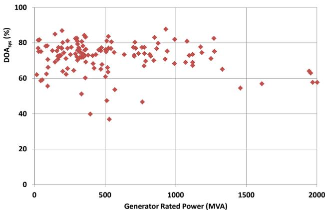
Fig. 5. Degree of asymmetry of the system-source short-circuit breaking current as a function of generator rated power
