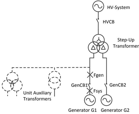
Fig. 2. Power station layout with two generators connected to a three-winding step-up transformer
