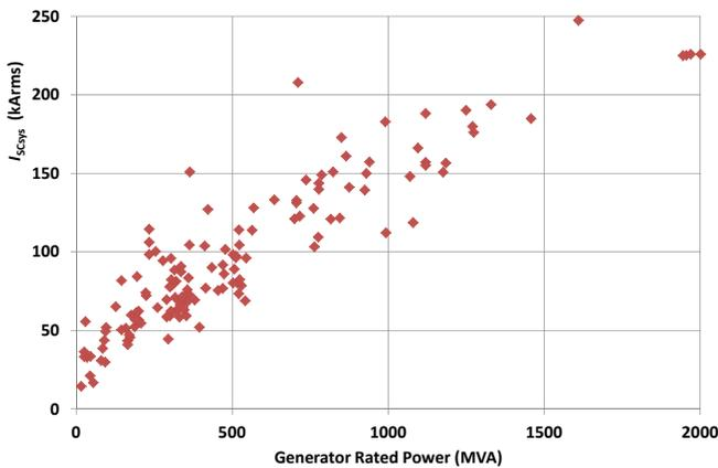
Fig. 4. A.C. component of the system-source short-circuit breaking current as a function of generator rated power
