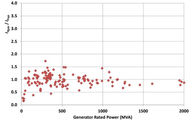
Fig. 9. Ratio of the peak value of the generator-source short-circuit current to the peak value of the system-source short-circuit current as a function of generator rated power
