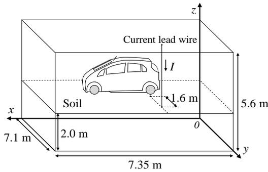
Fig. 3. Simulation setup in the case of a nearby lightning stroke.
