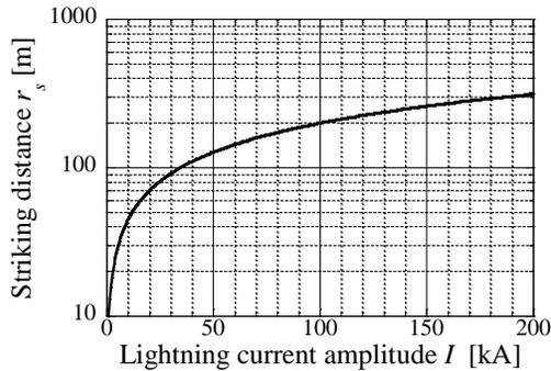
Fig. 4. Striking distance vs. lightning current amplitude.
