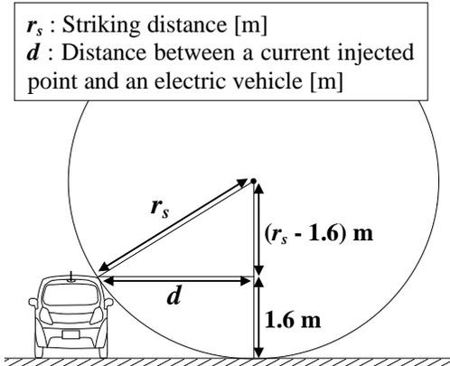
Fig. 5. Rolling sphere method.
