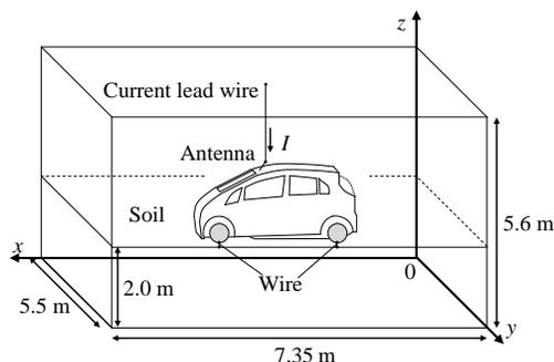
Fig. 1. Simulation setup in the case of a direct lightning stroke.
