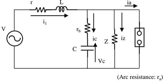
Fig. 9. SLF simplified calculation circuit
