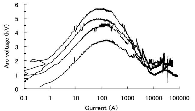
Fig. 3. Measurement result, the relation between current and arc voltage of 550kV model circuit breaker
