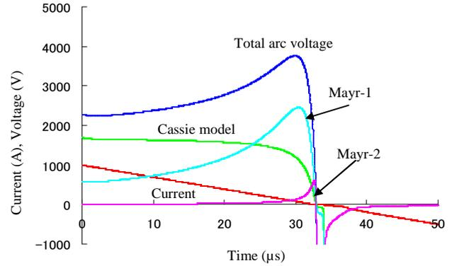
(b) 550kV - 63kA - 90%, 60Hz, interruption failed
