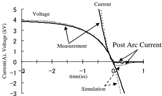
Fig. 2. Comparison between measured and simulated waveforms for 300kV SF<sub>6</sub> gas model circuit breaker
