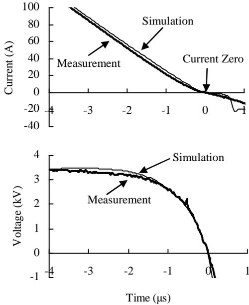
Fig. 4. Comparison between measured and simulated waveforms for 550kV SF<sub>6</sub> gas model circuit breaker, case of interruption failure
