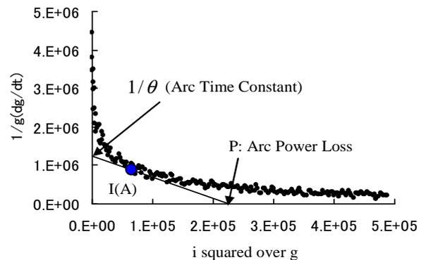
Fig. 6. Explanation for calculation of Mayr arc time constant in  $i^2/g -1/g dg/dt$
