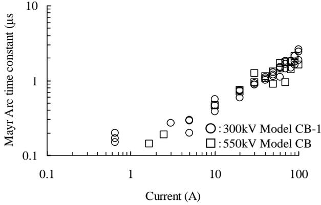
Fig. 7. Mayr arc time constants of 300kV model CB-1 and 550kV model CB
