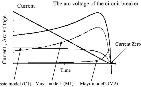
Fig. 1. Explanation of serially connected three arc models
