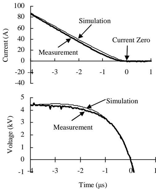
Fig. 5. Comparison between measured and simulated waveforms for 550kV SF<sub>6</sub> gas model circuit breaker, case of interruption successful
