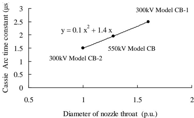
Fig. 8. Relation between Cassie arc time constants and diameter of nozzle throat
