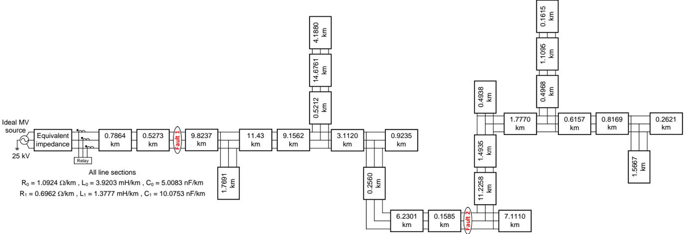
b) Distribution test system – 25 kV
