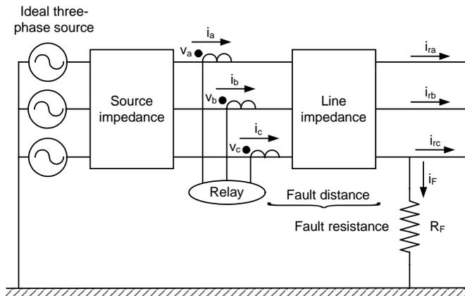
Fig. 1. Equivalent circuit of the faulted system.
