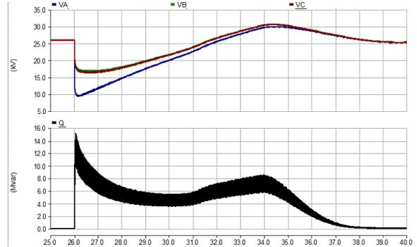
Fig. 6 Black Start Generator Low Voltage Bus Voltage Sag and Transformer Reactive Demand during Energization of Generator Step up Transformer
