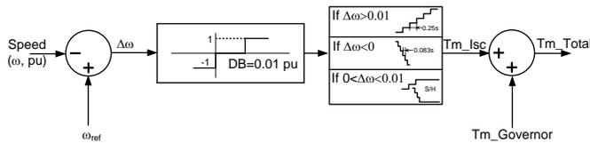
Fig. 1 – Implementation of Isochronous Controller used in the Studies
