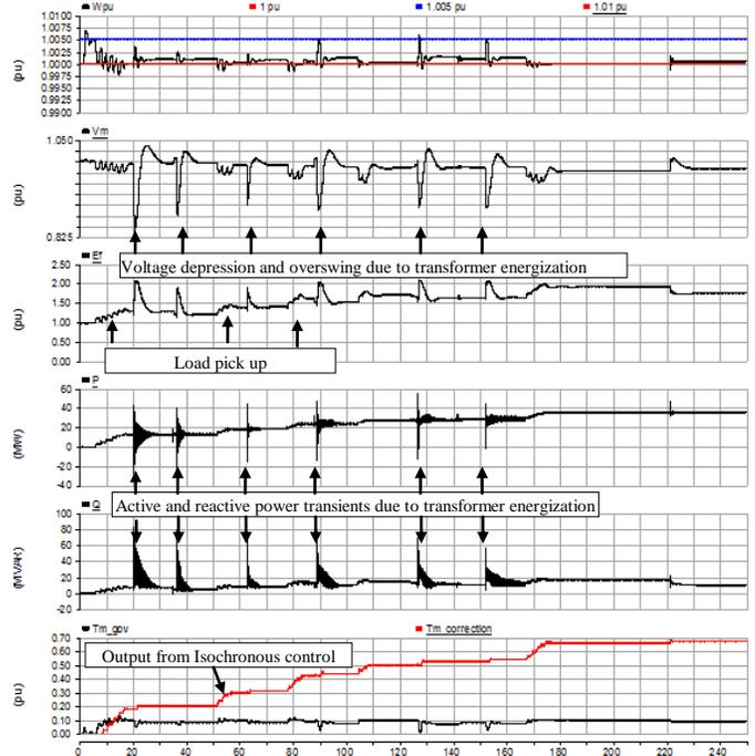
Fig. 4 Step-by-step Energization of the Island 1 with Black Start Generators loaded to 60% of Rated Capacity with Remanence
