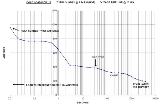
Fig. 2 - Example of Load Pickup after Outages for Summer Conditions [6]
