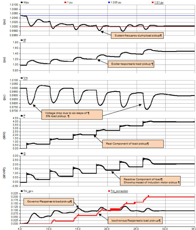
Fig. 5 Load Pick-up at Island 2 black start generator
