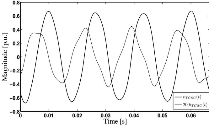
Fig. 5. Voltage at TCSC's terminals and current into the TCSC.
