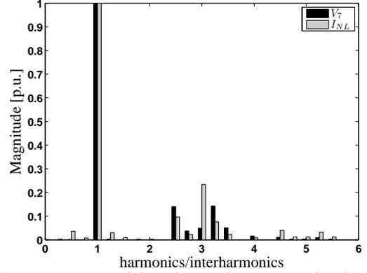
Fig. 9. Frequency content of the voltage and current entering the nonlinear load at bus 7.
