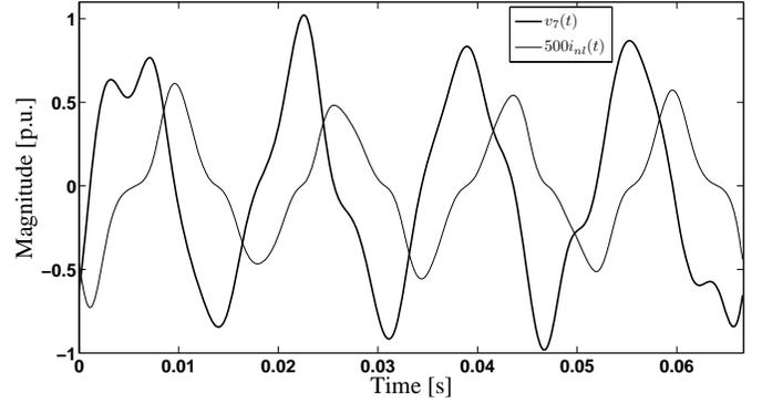
Fig. 8. Waveforms of voltage and current at bus 7.
