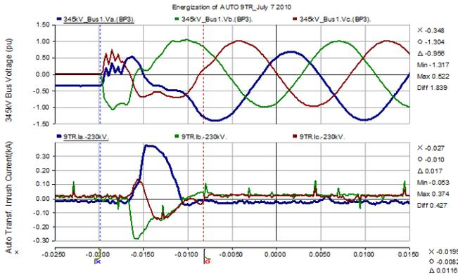
Fig. 10 Field Energization of 230/345 kV auto-transformer after pre-insertion resistor insertion time was adjusted (July 7 2010).
