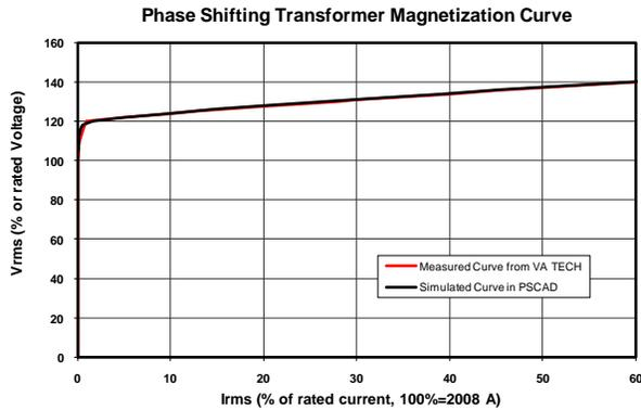
Fig. 2 Measured and modeled PST saturation characteristic
