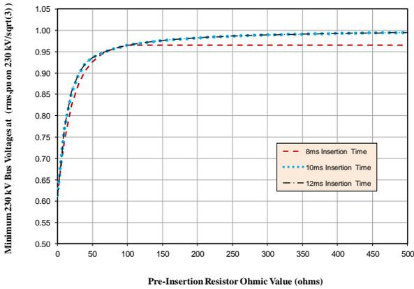
Fig. 4 Effect of ohmic value of pre-insertion resistor (Energize at Phase A Voltage Zero Crossing, 0.8 pu Remanence on Phase A)
