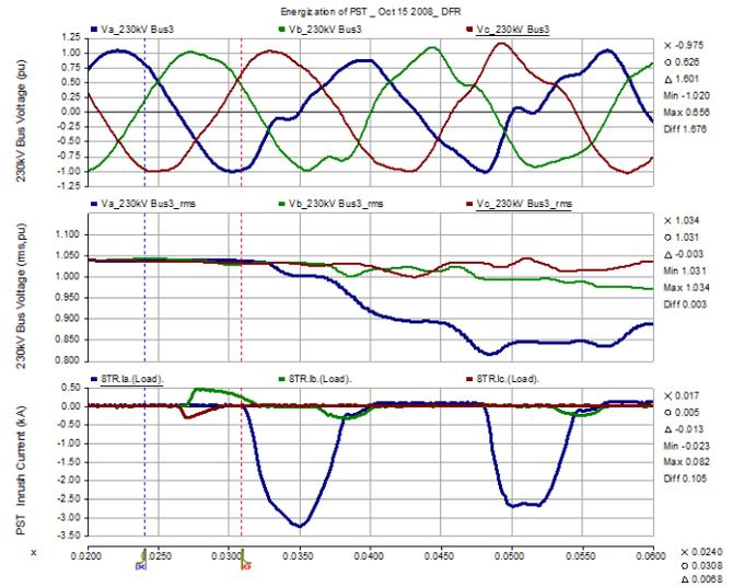
Fig. 7 Energization of phase shifting transformer with pre-insertion resistor insufficient insertion time of about 6.8 ms on Oct 15, 2008.
