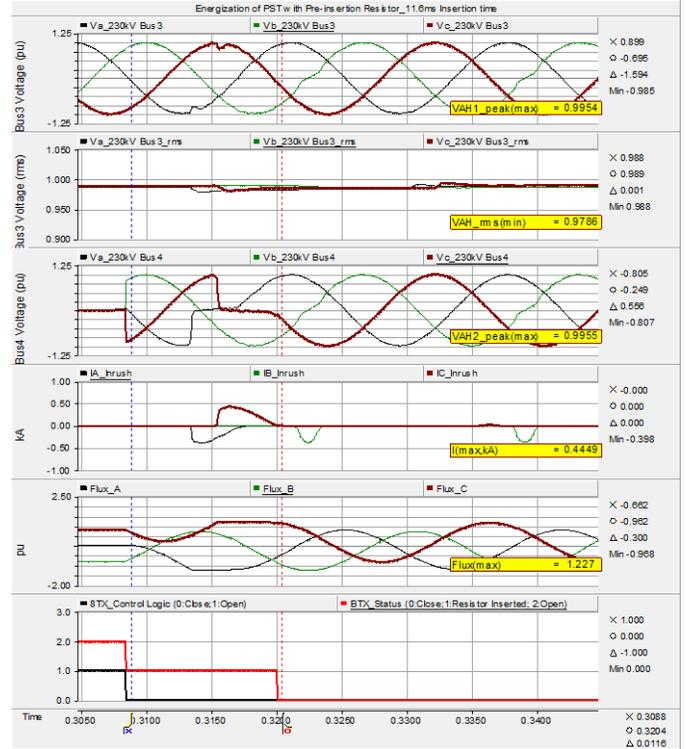
Fig. 11 PSCAD/EMDC Simulation of Energizing phase shifting transformer with 400 ohm pre-insertion resistor and 11 ms insertion time
