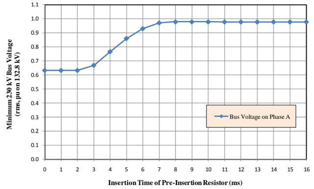
(b) Minimum Voltage at 230 kV Bus
