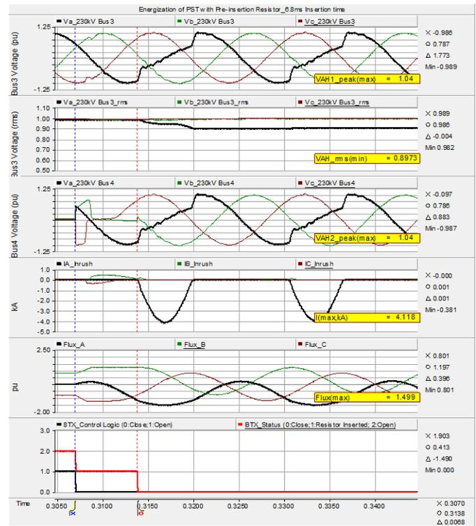
Fig. 8 PSCAD/EMDC Simulation Showing Energization of phase shifting transformer with 400 ohm pre-insertion resistor and 6.8 ms insertion time
