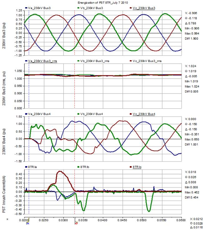
Fig. 9 Field Energization of phase shifting transformer (PST) after pre-insertion resistor insertion time was adjusted (July 7 2010)
