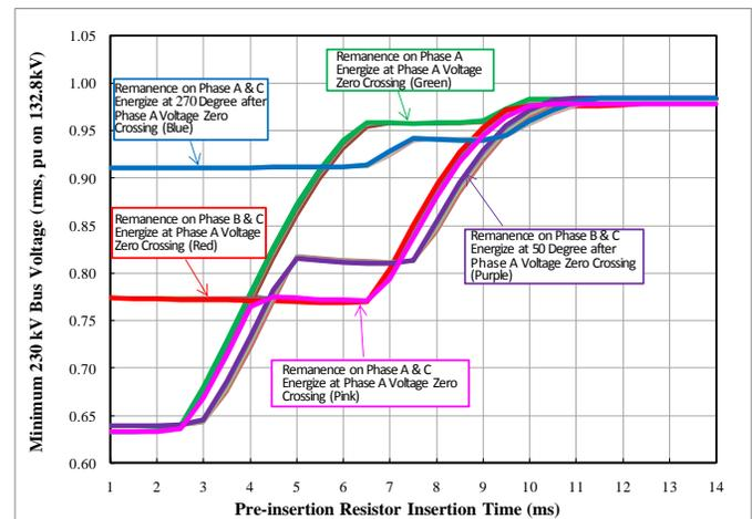
Fig. 6 Effects of Remanent Flux Conditions and Energization Instants
