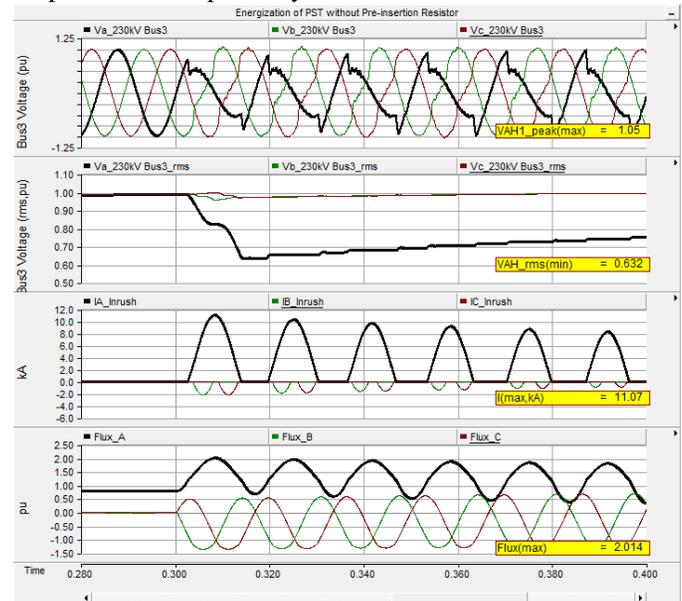
Fig. 3 Simulated waveforms for Energization of phase shifting transformer without pre-insertion resistors (Energized at Phase A voltage zero with 0.8 pu remanent flux)
