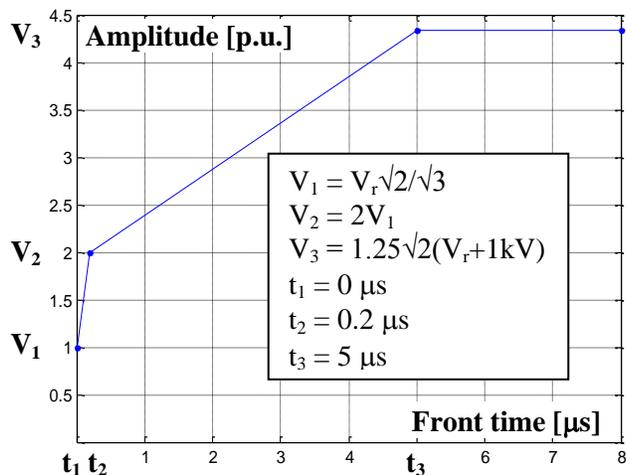
Fig. 1. Machine impulse withstand envelope [4]
