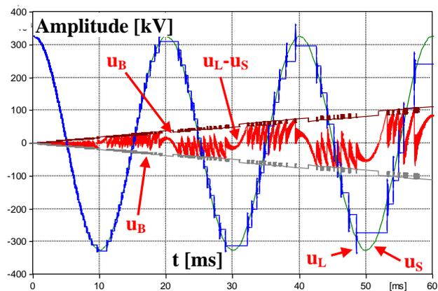
Fig. 2. VFT entire process, first 60 ms for opening operation;  $u_S$  – disconnector source side voltage,  $u_L$  – disconnector load side voltage,  $u_B$  – breakdown voltage,  $u_S-u_L$  – voltage across the contacts of disconnector
