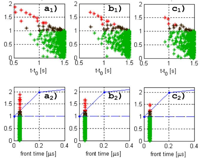
Fig. 6. Dot-plots of the VFT overvoltage for closing operation, different levels of trapped charge; a<sub>1-2</sub>) -1 p.u., b<sub>1-2</sub>) -0.6 p.u., c<sub>1-2</sub>) -0.2 p.u.; a<sub>1</sub>-c<sub>1</sub>) VFT overvoltage amplitude vs. time, a<sub>2</sub>-c<sub>2</sub>) VFT overvoltage amplitude and front time over the withstand envelope
