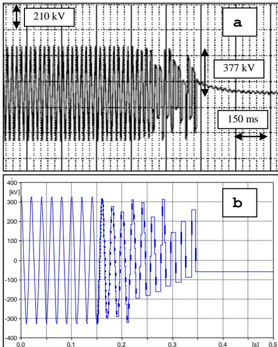
Fig. 3. Simulation results vs. measurements in Test Duty 1 for opening operation, load side voltage: a) measurements, b) simulation
