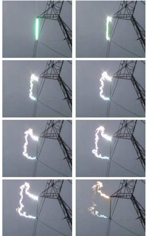
Fig. 4. Images of the test of arc rating 200 A_{rms} .
