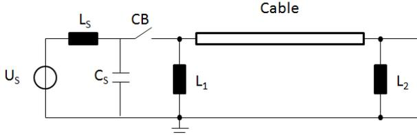
Fig. 4. Resonance between cable and shunt reactors when cable is switched off
