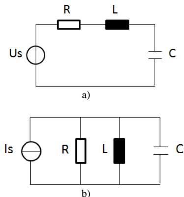
Fig. 1. Resonance Circuit Diagram; a) Series resonance, b) Parallel resonance
