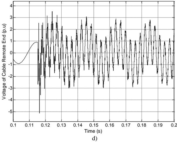
Fig. 5. Voltage of circuit breaker during cable switching. a) 0% ; b) 80% compensated; c) 90% compensated; d) Voltage of cable remote end after reclosing with cable 80% compensated.
