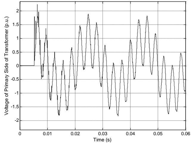
Fig. 7. Resonance between cable and transformer, together with shunt reactors.
