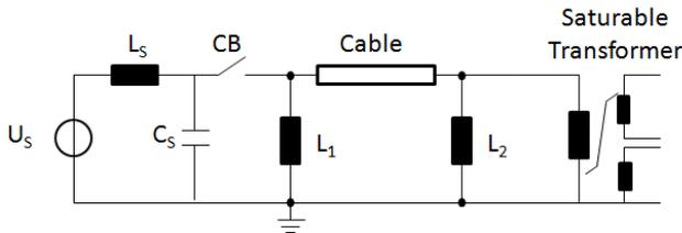
Fig. 6. Resonance between transformer and cable when transformer is being connected.
