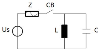
Fig. 2. Resonance example according to switching event in power system
