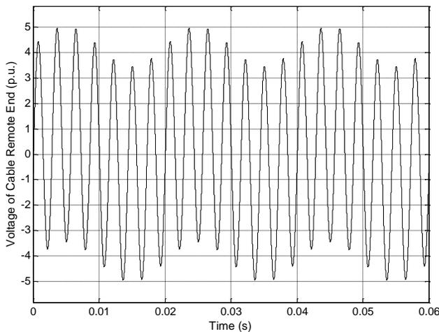
Fig. 9. Voltage of cable remote end caused by harmonic source
