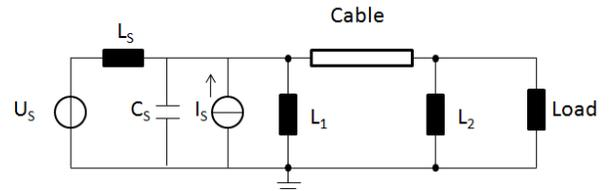
Fig. 8. Resonance caused by harmonic sources
