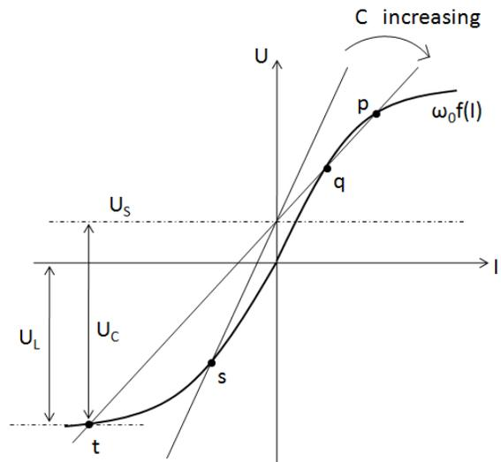
Fig. 3. Ferroresonance basic principle
