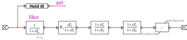
Fig. 4. IEEE PSS1A transfer function.  $P_e$  is filtered by the parameter  $T_6$
