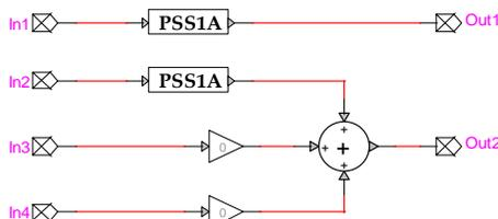
Fig. 2a. Structure of G(s) 4in-2out, connected with F(s) 2in-4out.
