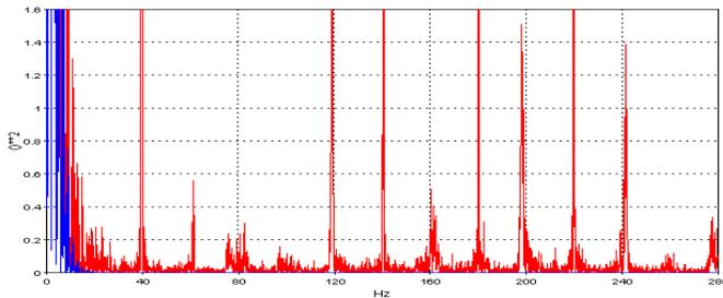
Fig. 5. Electrical power signals spectral energies: before (red) and after (blue) filtering.
