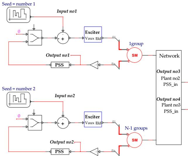
Fig. 1. EMTPTWorks. State-space set-up for open and closed linear analysis.
