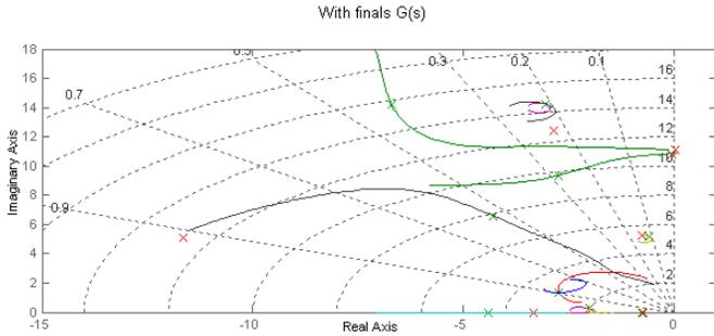
Fig.12 Root locus trajectories with  $G(s)$  gain varying 0 to 10. Gain=0 “red x”; gain=nominal “green x”. Top, initial parameters - bottom, final tuning.
