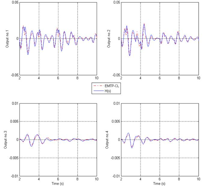
Fig. 7. Validation of  $H(s)$  with EMTP, PSS in close loop.
