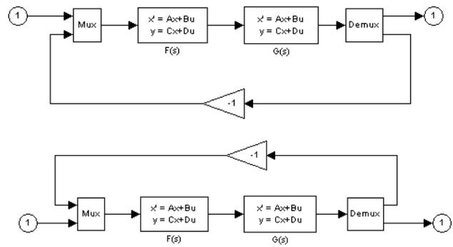
Fig.11. Two SISO transfer functions derived from a single MIMO H(s).
