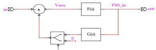
Fig. 2b. Schematic. State-space set-up for open and closed linear analysis.
