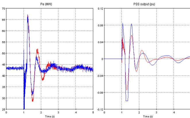
Fig. 13 Loss of line in EMTP. Initial (red) and after Optimization (blue).
