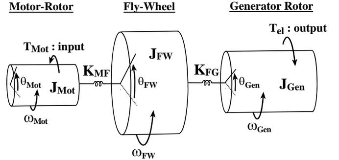
Fig. 4. Mass-spring model of the EZ3 shaft system
