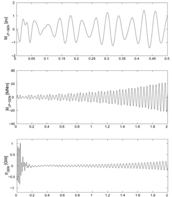
Fig. 8. SSR excitation in the Second Benchmark Model by a three-phase fault (clearing time 40 ms)
