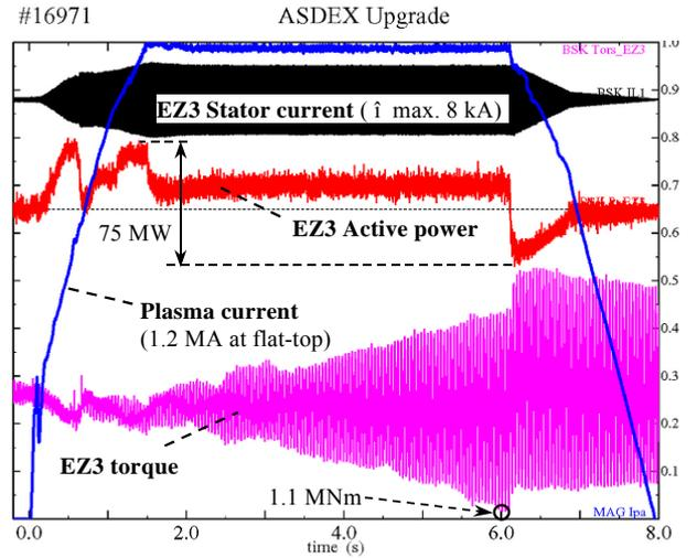
Fig. 5. Measured EZ3 generator current, active power and torque showing a torsional resonance excited by active power transients during AUG plasma experiment #16971
