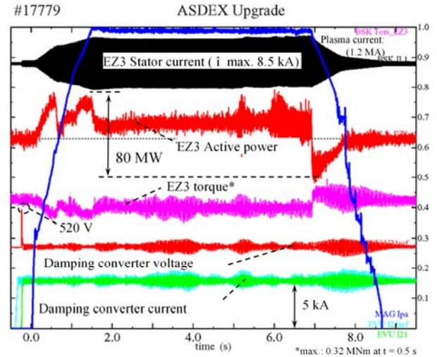
Fig. 6. Stabilization of the oscillating torque caused by a plasma experimental comparable to #16971 in using the EZ3 torque stabilizer at low operational gain (damping power < 1 MW)
