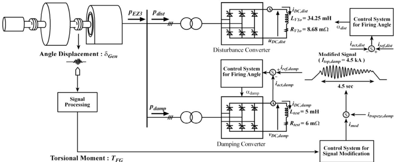
Fig. 3. Schematic of the test setup for excitation and damping of torsional oscillations in the assembly of generator EZ3
