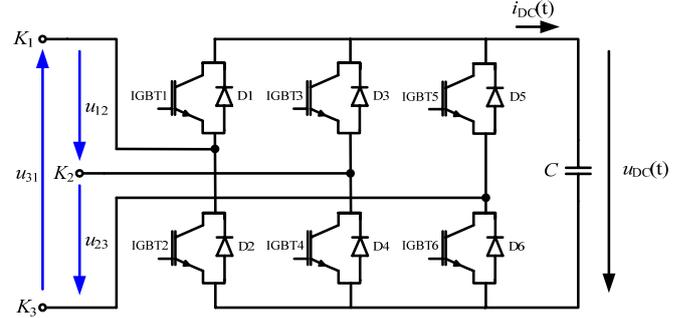
Fig. 10. Three phase self-commutated inverter with IGBTs and capacitive energy storage
