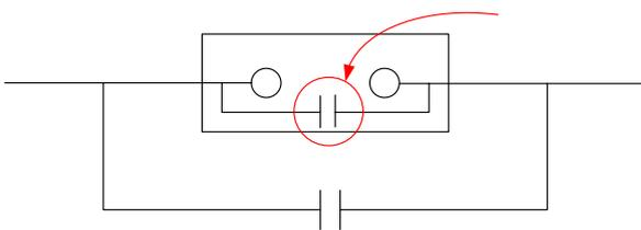
Fig. 9. 20000 pF capacitor parallel establishment with series reactor
