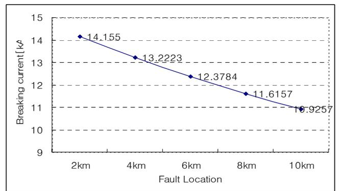
Fig. 6 - Breaking current by distance at SLF
