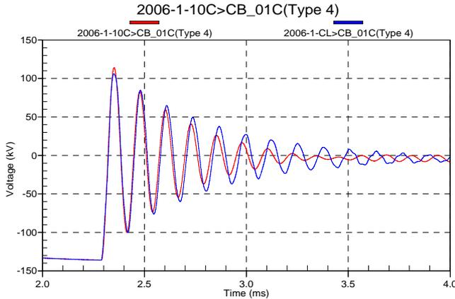
Fig. 8 - Waveform comparison at breaker/series reactor and 20000 pF capacitor parallel establishments
