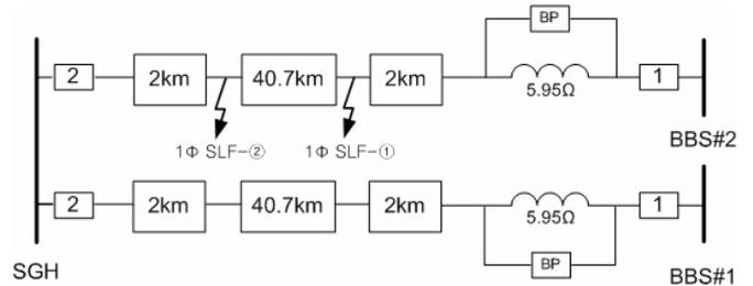
Fig. 2 - Simulation Condition on T/L
