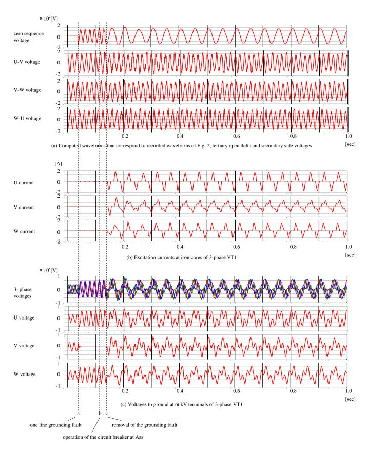
Fig. 4. Waveforms of ferro-resonance reproduced by the computation
