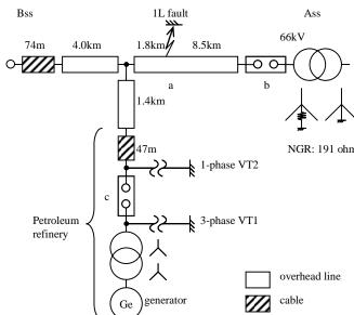
Fig. 1. Configuration of the power system where the ferro-resonance happed.
