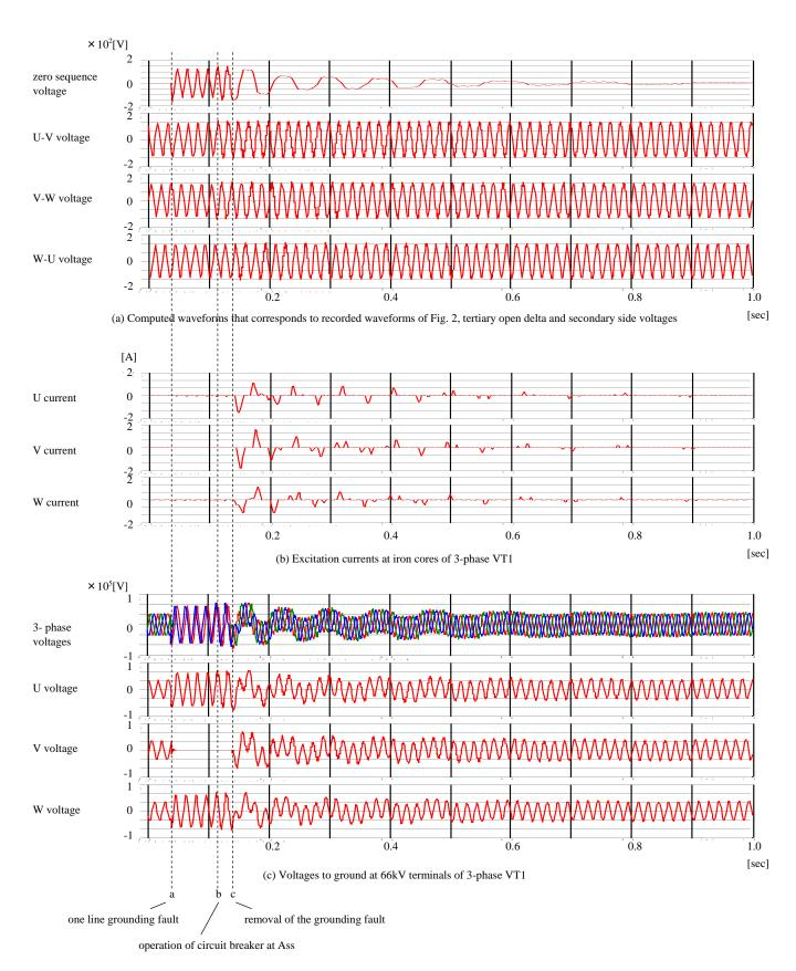
Fig. 5. Computed voltage waveforms without the single phase VT2, no generation of the ferro-resonance.
