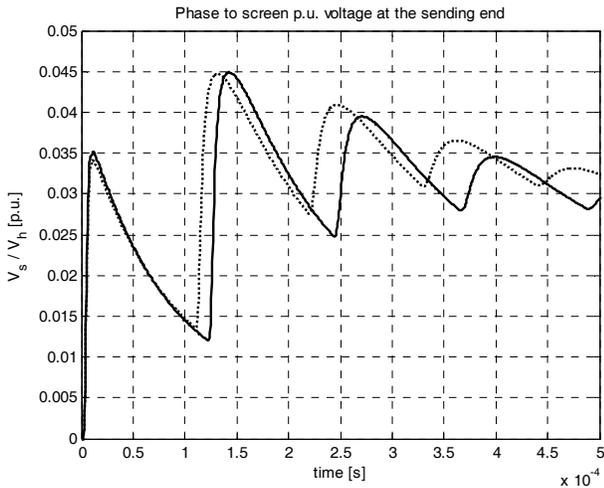
Fig. 5. Cable line voltage at the sending end in p.u. value of the maximum impinging voltage on a 20 kV cable line 10 km long for the 1.2/50  $\mu\text{s}$  impinging wave shapes when semiconductive layers are not taken into account (dashed lines) and 0.7 mm and 0.5 mm of inner and outer semiconductive layers respectively are considered (solid lines).
