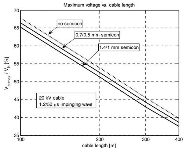
Fig. 7. Maximum voltage stemming on the cable / maximum impinging overvoltage ratio in percent on a 20 kV cable line vs. cable length for the 1.2/50  $\mu\text{s}$  impinging wave shape when no semiconductive layers, 0.7 mm/0.5 mm of inner/outer semiconductive layers thickness and 1.4 mm/1 mm of inner/outer semiconductive layers thickness are considered.
