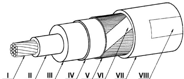
Fig. 2. Typical EPR cable formation: (I) conductor, (II) inner semiconductive layer, (III) insulation wall, (IV) outer semiconductive layer, (V) wire screen, (VI) equalizer tape, (VII) thermoplastic jacket, (VIII) stamping.
