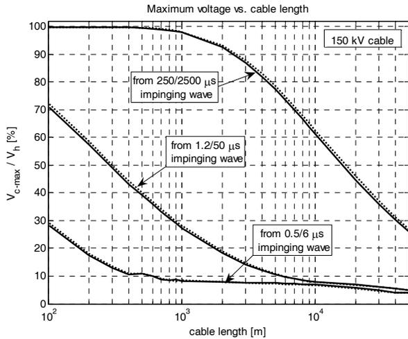
Fig. 8. Maximum voltage stemming on the cable / maximum impinging overvoltage ratio in percent on a 150 kV cable line vs. cable length for different impinging wave shapes when semiconductive layers are not taken into account (dashed lines) and 2 mm and 1 mm of inner and outer semiconductive layers respectively are considered (solid lines).
