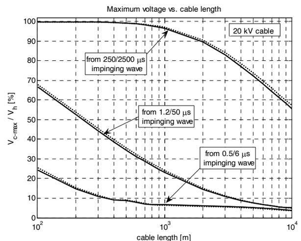
Fig. 3. Maximum voltage stemming from the cable / maximum impinging overvoltage ratio in percent on a 20 kV cable line vs. cable length for different impinging wave shapes when semiconductive layers are disregarded (dashed lines) and 0.7 mm and 0.5 mm of inner and outer semiconductive layers respectively are considered (solid lines).
