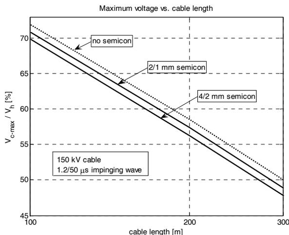
Fig. 9. Maximum voltage stemming on the cable / maximum impinging overvoltage ratio in percent on a 150 kV cable line vs. cable length for the 1.2/50  $\mu$ s impinging wave shape when no semiconductive layers, 2 mm/1 mm of inner/outer semiconductive layers thickness and 4 mm/2 mm of inner/outer semiconductive layers thickness are considered.
