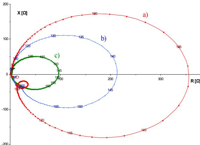
Fig. 8. Phase A diagram of the complex impedance of the network calculated at bus A with the prospective link (see Fig. 1). The numbers near to the points marked are frequencies in Hertz. a) Minimum load with "weak" network; b) minimum load; c) maximum load
