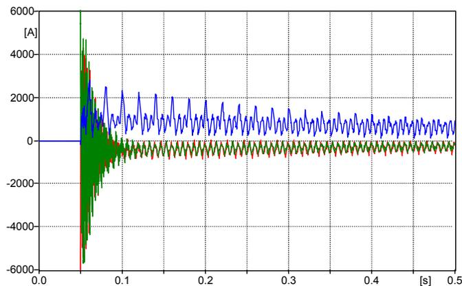
Fig. 12. Phase currents, in case of no-load energization of the 2nd circuit of the new prospective link from bus A (see Fig. 1) with the system at minimum load (case b of Fig. 8). Saturation voltage of the shunt reactors equal to 150% of their rated voltage
