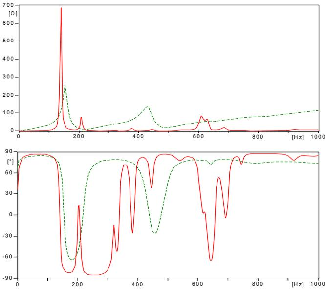
Fig. 7. Phase A driving point impedance, in modulus and phase, calculated at bus A of the Fig.1 system at no-load, with the prospective link in case of positive (solid) and zero (dashed) sequence current excitation
