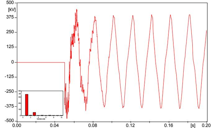
Fig.9. Phase-to-Gr overvoltage and FFT analysis (initial time 0.18 s, final time 0.20 s), in A phase for the no-load energization of the prospective link from bus A (see Fig. 1) with the system at minimum load (case b of Fig. 8). Saturation voltage of the shunt reactors equal to 125% of their rated voltage
