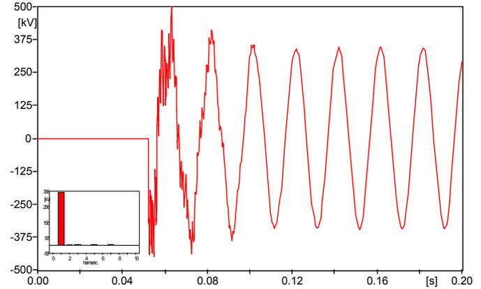
Fig.13. Phase-to-Gr overvoltage and FFT analysis (initial time 0.18 s, final time 0.20 s), in A phase at bus A for the no-load energization of the system with the prospective link. Synchronized switching simulated. Saturation voltage of the shunt reactors equal to 125% of their rated voltage
