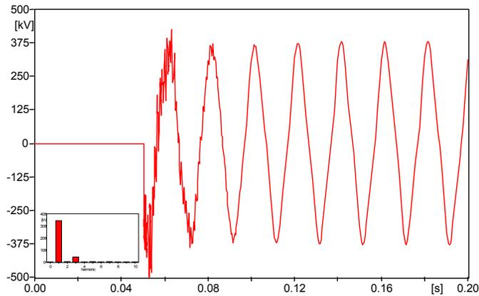
Fig.11. Phase-to-Gr overvoltage and FFT analysis (initial time 0.18 s, final time 0.20 s), in A phase for the no-load energization of the prospective link from bus A (see Fig. 1) with the system at minimum load (case b of Fig. 8). Saturation voltage of the shunt reactors equal to 150% of their rated voltage
