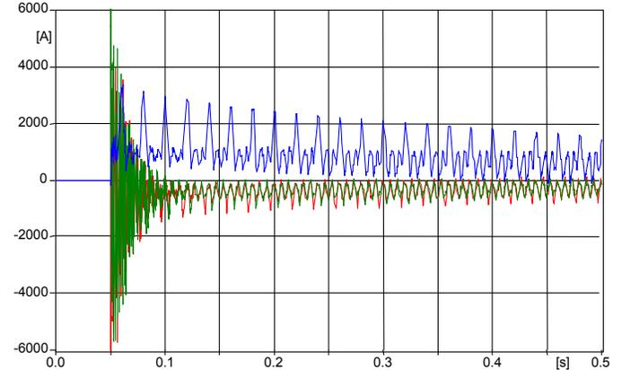
Fig.10. Phase currents, in case of no-load energization of the 2nd circuit of the new prospective link from bus A (see Fig. 1) with the system at minimum load (case b of Fig. 8). Saturation voltage of the shunt reactors equal to 125% of their rated voltage
