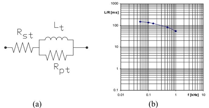
Fig. 4. Equivalent circuit of the transformer series impedance (a) and assumed time constant for the leakage inductance of a 370 MVA 20/240 kV step-up transformer (b)
