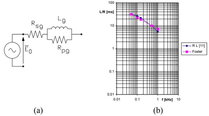
Fig. 3. Frequency domain synchronous generator equivalent circuit of one phase (a) and time constant  $L/R$  of the equivalent R-L series circuit (b)
