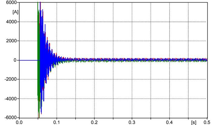
Fig.14. Phase currents, in case of no-load energization of the 2nd circuit of the new prospective link from bus A (see Fig. 1) with the system at minimum load (case b of Fig. 8). Synchronized switching simulated. Saturation voltage of the shunt reactors equal to 125% of their rated voltage
