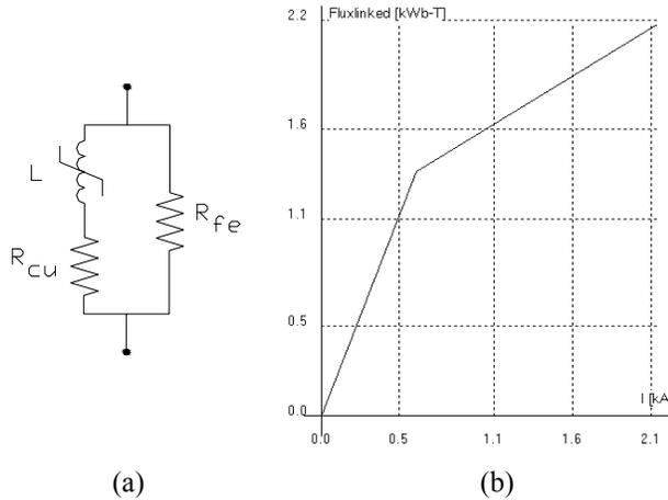
Fig. 2. 420 kV 250/3 Mvar shunt reactor model of one phase (a) and saturation curve with saturation voltage at 125% of rated voltage (b)
