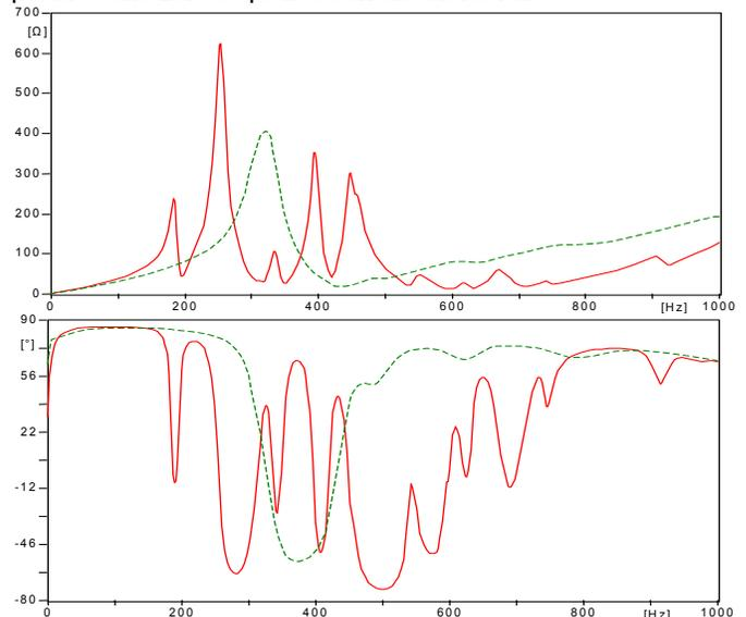
Fig. 6. Phase A driving point impedance, in modulus and phase, calculated at bus A of the Fig.1 system at no-load, without the prospective link in case of positive (solid) and zero (dashed) sequence current excitation
