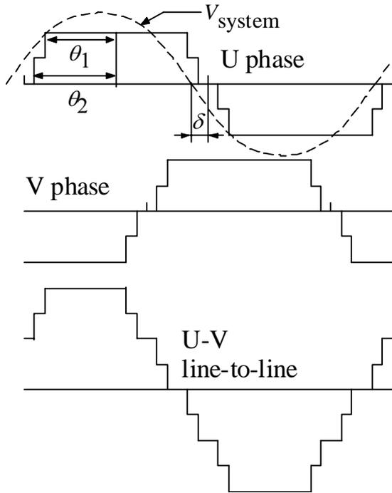
Fig.2 Output voltage of 5 level converter
