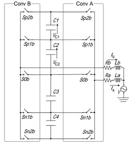
Fig.8 ATP simulation model of double converter circuit in one line diagram
