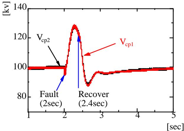
(b) DC capacitor voltage
