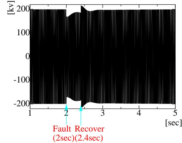
(a) AC system voltage at installation point
