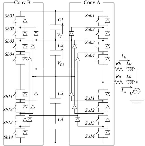
Fig.3 Double converter configuration of 5 level converter
