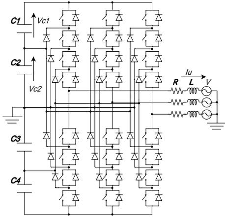
Fig.1 Circuit of 5 level converter
