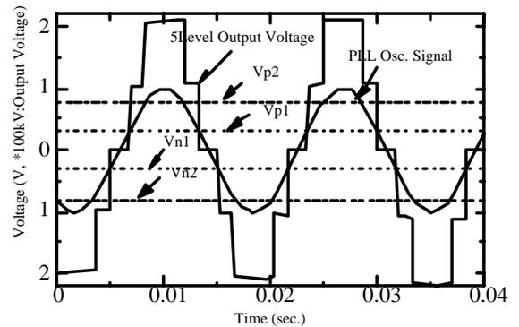
Fig.4 Control signal and output voltage of 5 level converter (PLL Osc. signal: Sine Wave Phase Shifted to AC system; Vp2, Vp1, Vn1, Vn2: Reference Voltage for Pulse Width)
