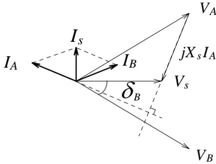
Fig.7 Phasor diagram of reactive power control system using phase control
