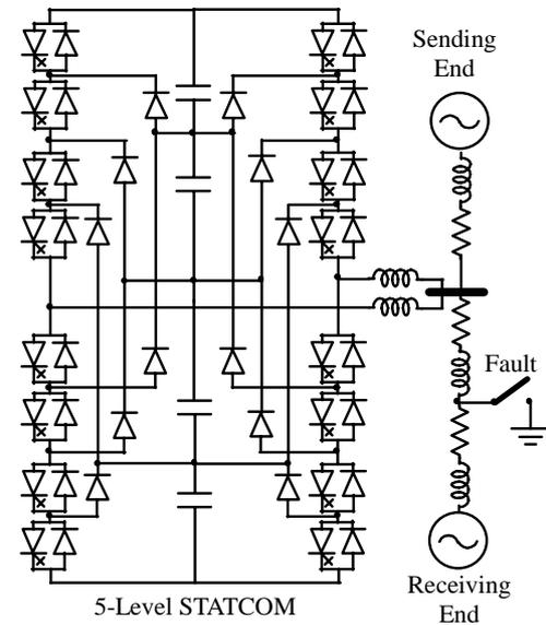
Fig.9 Simulation system with STATCOM installed at the mid-point of long ac transmission line in one line diagram
