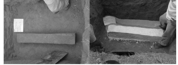
Figure 2 – Cuboid sample cut and covered with paraffin and net (photo: sample 3 – Cachoeira Paulista – 01/08/2002)
