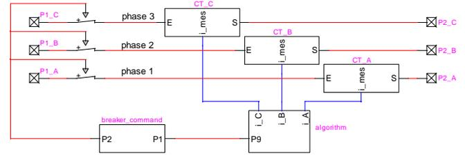
Fig. 2. Protective relay with the three CTs, the algorithm and the breaker's command.
