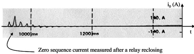
Fig. 7. instantaneous zero sequence current measured by a relay after a reclosing without fault. The effect of the inrush current clearly appears on these on-site registered data.
