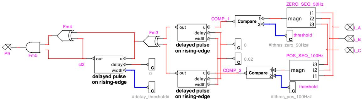
Fig. 4. Algorithm to discriminate an inrush current. The input parameters are  $I_{thres\_pos\_100Hz}$ ,  $I_{thres\_zero\_50Hz}$  and  $delay\_threshold$ . In the present paper the parameters values are respectively: 10 mA, 10 mA and 2 ms.
