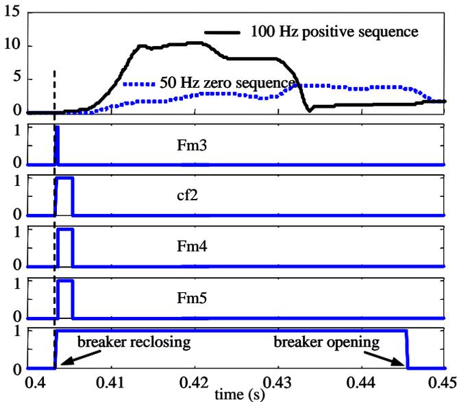
Fig. 8. Command signals generated by the algorithm. Phasors' amplitudes of the zero and positive sequences currents are in Ampere. Pulse for Fm5 → the breaker is re-opened with a 40 ms breaker delay
