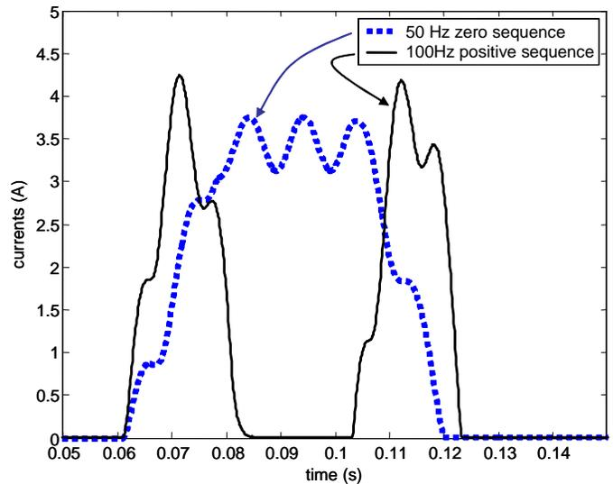
Fig. 10. 50 Hz zero sequence and 100 Hz positive sequence during the fault. The currents are calculated through a 20 ms width window.
