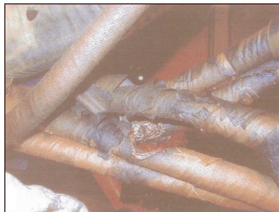
Fig.1: Flashover between tapping leads
