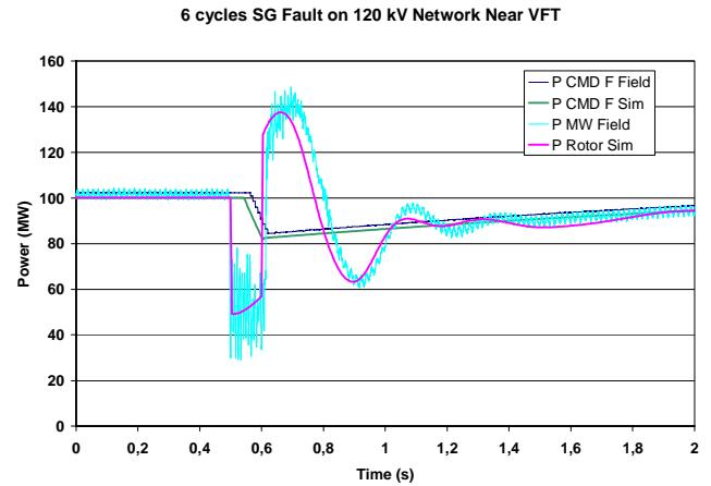
Fig. 9. Power Transfer Through the VFT During a Single Line to Ground Fault - Comparison Between Field Measurements and PSS/e Simulation.
