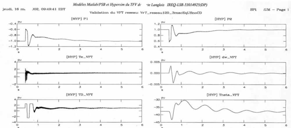
Fig 12 – Hypersim simulation results for VFT behavior after a 3 phase fault at Langlois 120 kV (HQ side)
