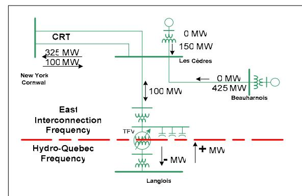
Fig. 2. Normal Operating System Configuration for Power Transfers Between HQ and NY
