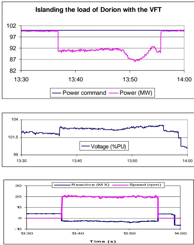
Figure 4-Local load at Dorion substation fed radially through the new Langlois VFT installation
