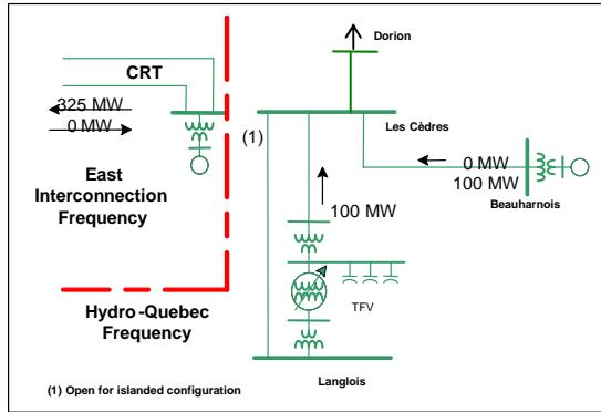
Fig. 3. Special Configuration for VFT operation with Power Transfer on HQ system only.
