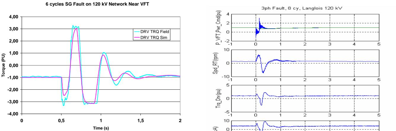
Fig. 10. VFT Torque During a Single Line to Ground Fault - Comparison Between Field measurements and PSS/e simulation
