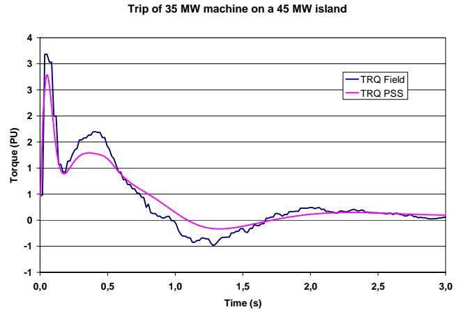
Fig. 8. Variation in Applied Torque on the VFT after Generator Trip - Comparison between Field Measurements and PSS/e Simulation.
