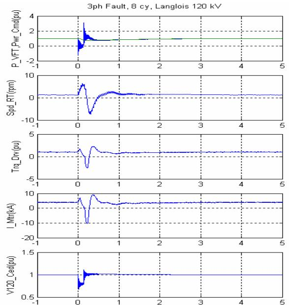
Fig. 11. Results from dynamic performance study for 3 phase fault at Langlois 120 kV on HQ side
