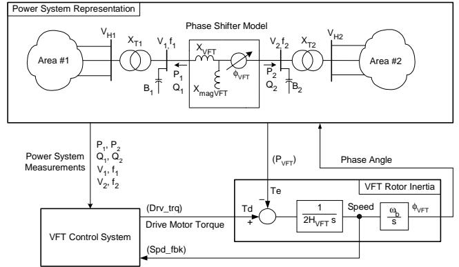
Fig 5: VFT Representation for Load Flow and Stability System Simulation
