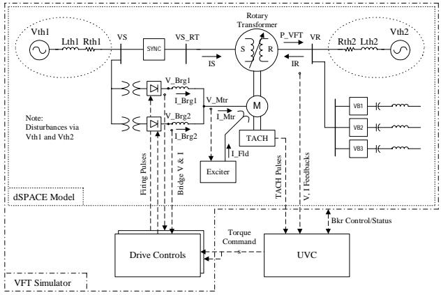
Fig 6. Overview of VFT Simulator Control Interfaces
