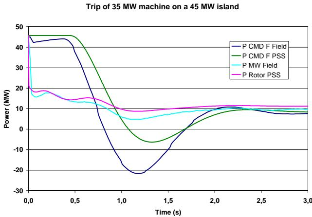
Fig. 7. Dynamic Behavior of the VFT after the trip of a 35 MW machine on a 45 MW island.
