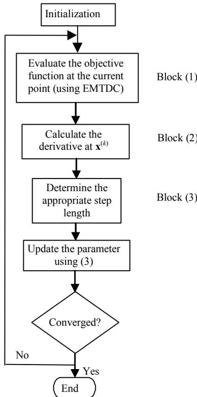
Fig. 2. Interface between the optimization algorithm and transient simulation
