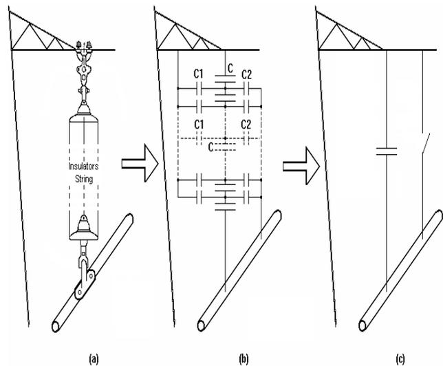
Figure # 5. Model used for string of insulator up 230 kV.
