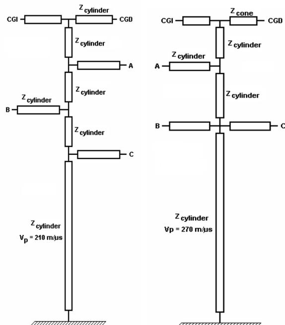
Figure # 6. Models used for tower and pole up 230 kV.
