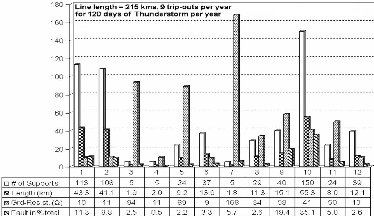
Figure # 7. Line forced outages rate for initial condition of footing resistance.
