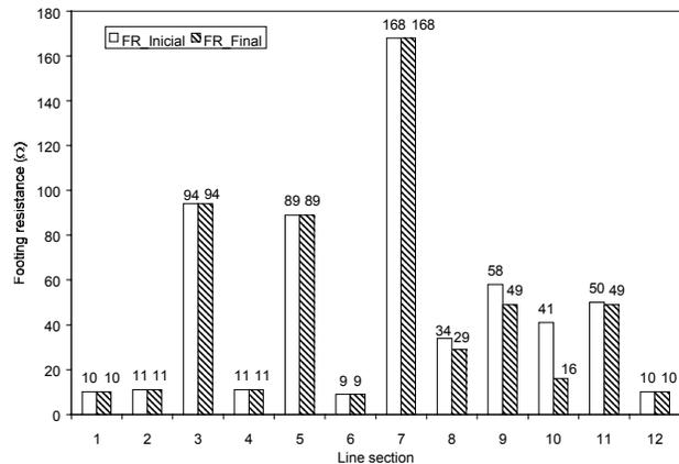
Figure # 3. Footing resistance measurements result along line Las Claritas–Santa Elena up 230 kV.
