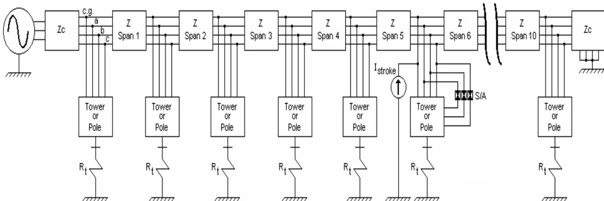
Figure # 4. Outline model used in ATP of the line up 230 kV.
