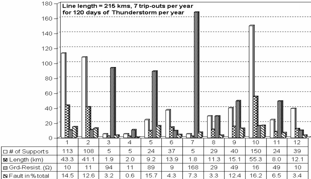
Figure # 8. Line forced outages rate for final condition of footing resistance.
