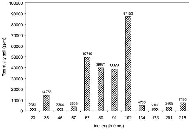
Figure # 1. Resistivity soil measurements result along line Las Claritas–Santa Elena up 230 kV.
