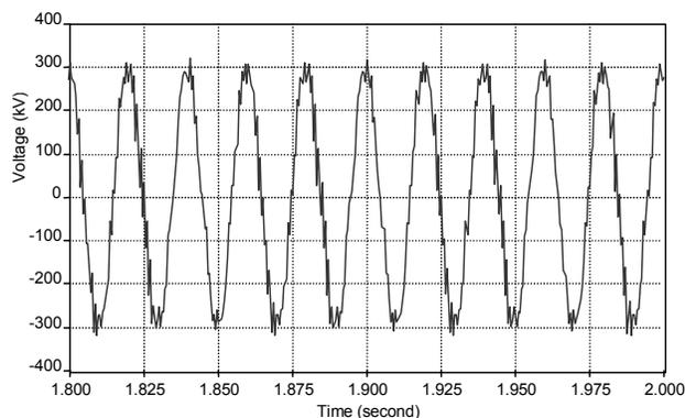
Fig. 7: Simulation Results – with Mitigation Measures for resonance over-voltage
