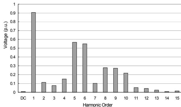
Fig. 3: Fourier Analysis of Resonance Over-voltage in figure 2
