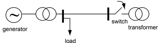
Fig. 1: Energizing a No-load Transformer
