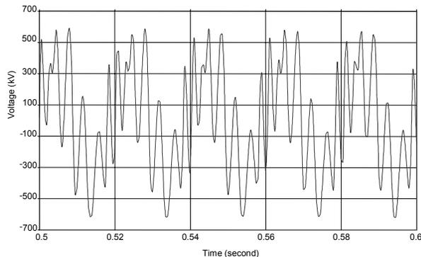
Fig. 2: Recorded waveform of Resonance Over-voltage
