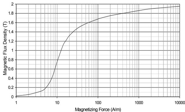
Fig. 4: A typical B-H curve of transformers
