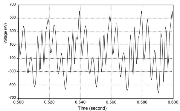
Fig. 5: Simulation Results – Reproduction of the recorded Resonance Over-voltage as compared with Fig. 2
