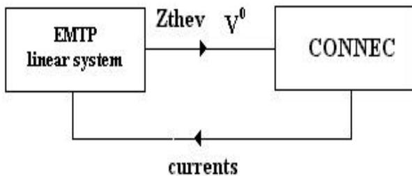
Fig. 1. Subroutine CONNEC and its interface with the main program.
