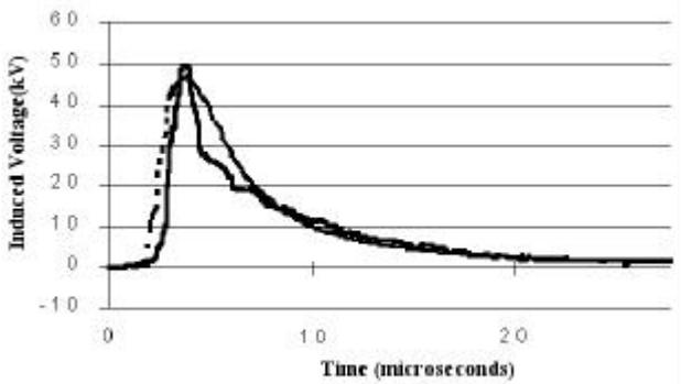
Fig. 4. Induced voltage as a function of time. Induced voltage from EMTP-Rusck (dashed line) and induced voltage from measurements (solid line) for lightning flash 9305 using data from Jankov [7].
