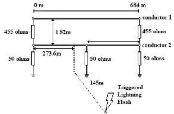
Fig. 2. Phase conductor 1 and neutral conductor 2, and discharge configuration.
