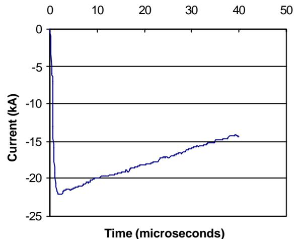
Fig. 3. Typical stroke current waveform.
