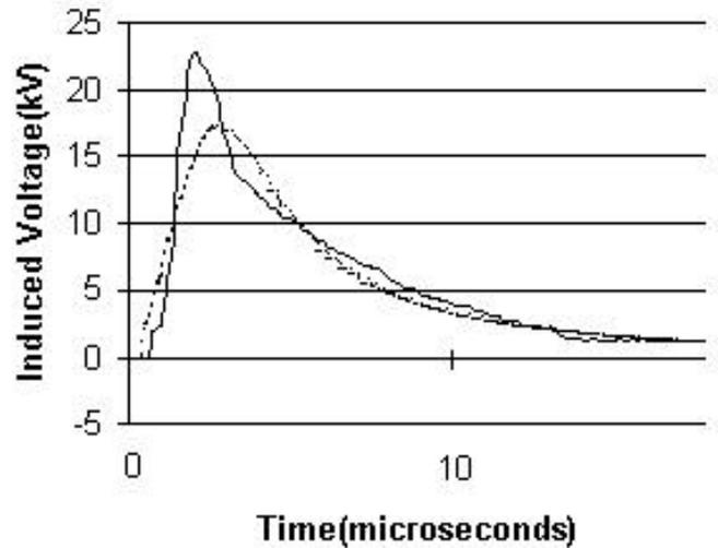
Fig. 6. Induced voltage as a function of time. Induced voltage from EMTP-Rusck (dashed line) and induced voltage from measurements (solid line) for lightning flash 9313-2 using data from Jankov [7].
