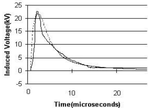
Fig. 7. Induced voltage as a function of time. Induced voltage from EMTP-Rusck (dashed line) and induced voltage from measurements (solid line) for lightning flash 9313-2 using data from Jankov [7], but with front time of  $1\mu\text{s}$  from digitized data.
