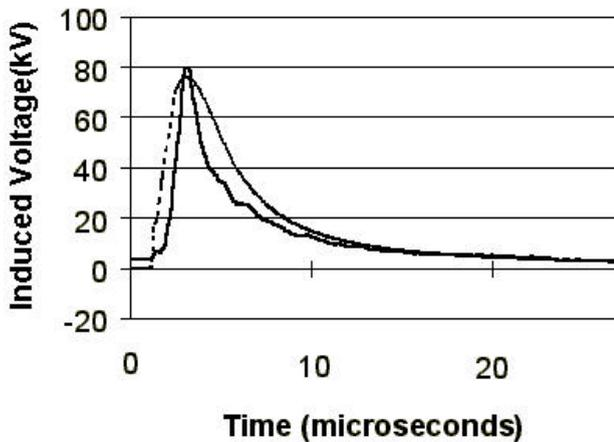
Fig. 5. Induced voltage as a function of time. Induced voltage from EMTP-Rusck (dashed line) and induced voltage from measurements (solid line) for lightning flash 9306 using data from Jankov [7].
