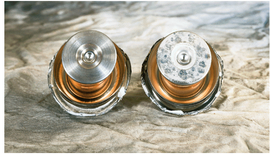
Figure 10b. A New Contact and Contact after 2,500 Capacitor Switching Operations
