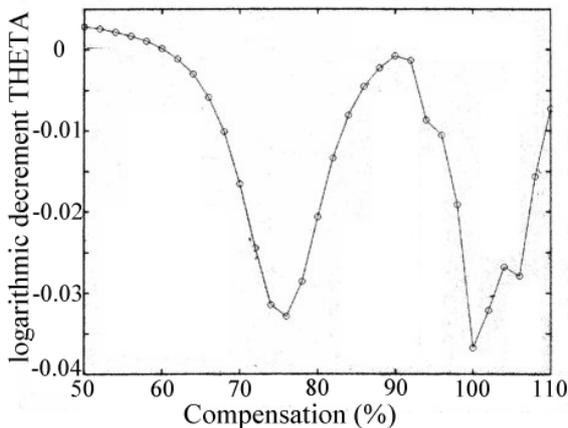
Fig. 5. Logarithmic damping decrement after 1-phase fault
