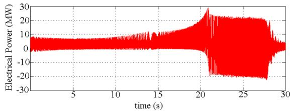
Fig. 10.: Calculated time-function of the electrical power fed by faulty slip ring machine
