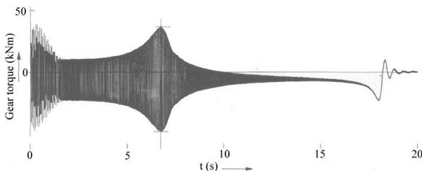
Fig. 8.: Calculated gear torque
