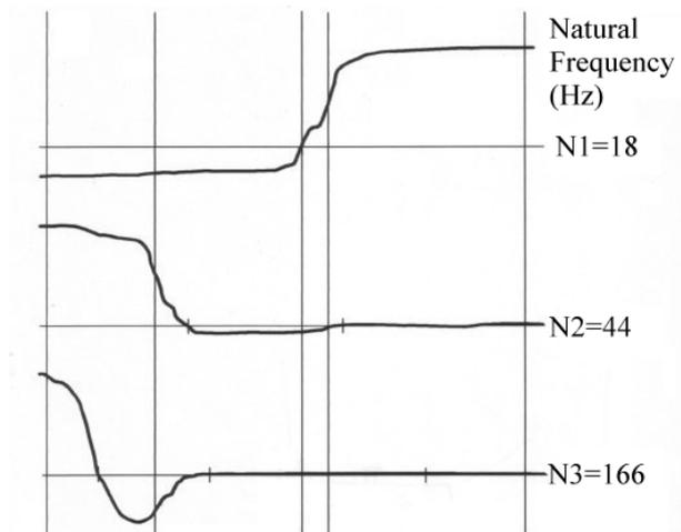
Fig. 3: Modes of the steam turbine generator shaft system
