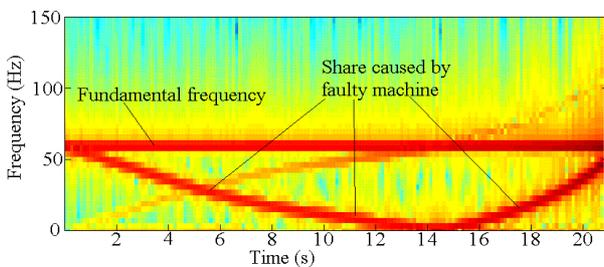
Fig. 11.: Calculated Spectra of current of a faulty slip ring machine during running up
