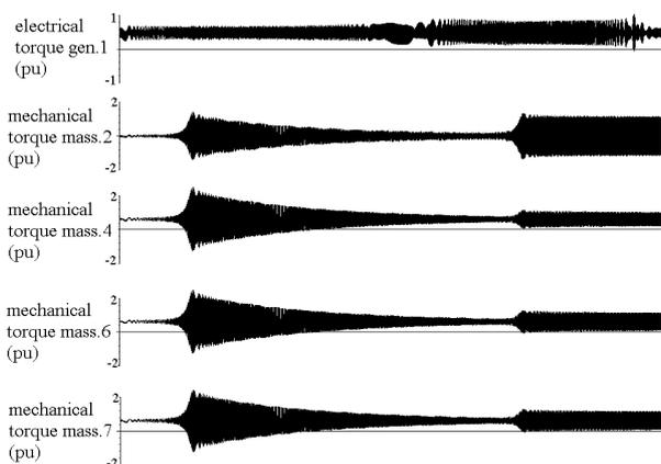
Fig. 12: Electrical and mechanical torque
