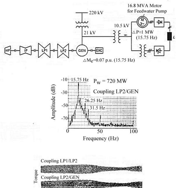
Fig. 6. Subsynchronous torsional resonance of a 775 MW turbine generator due to feedback from a thyristor cascade
