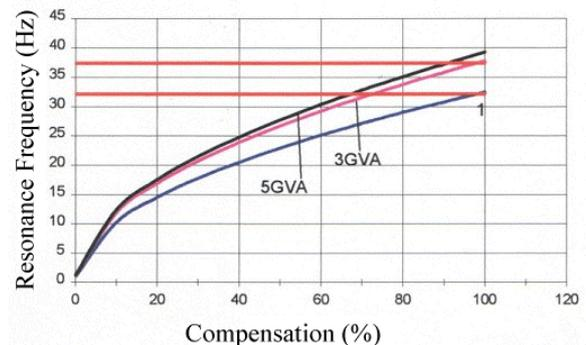
Fig. 4. Resonance frequencies of the main system
