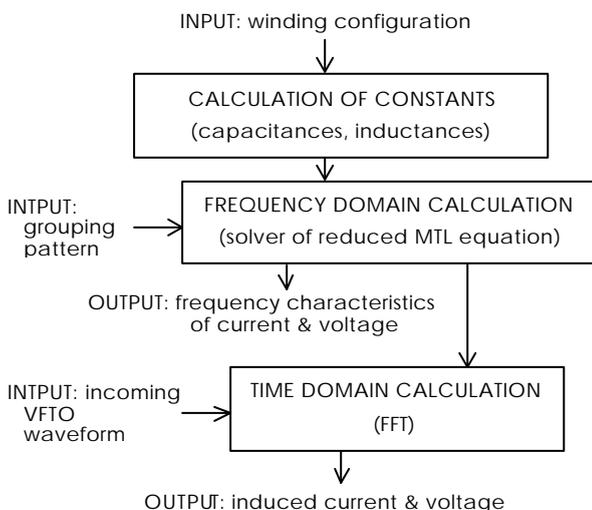
Fig. 12. Flow to calculate high frequency characteristics of transformer using MTL model.
