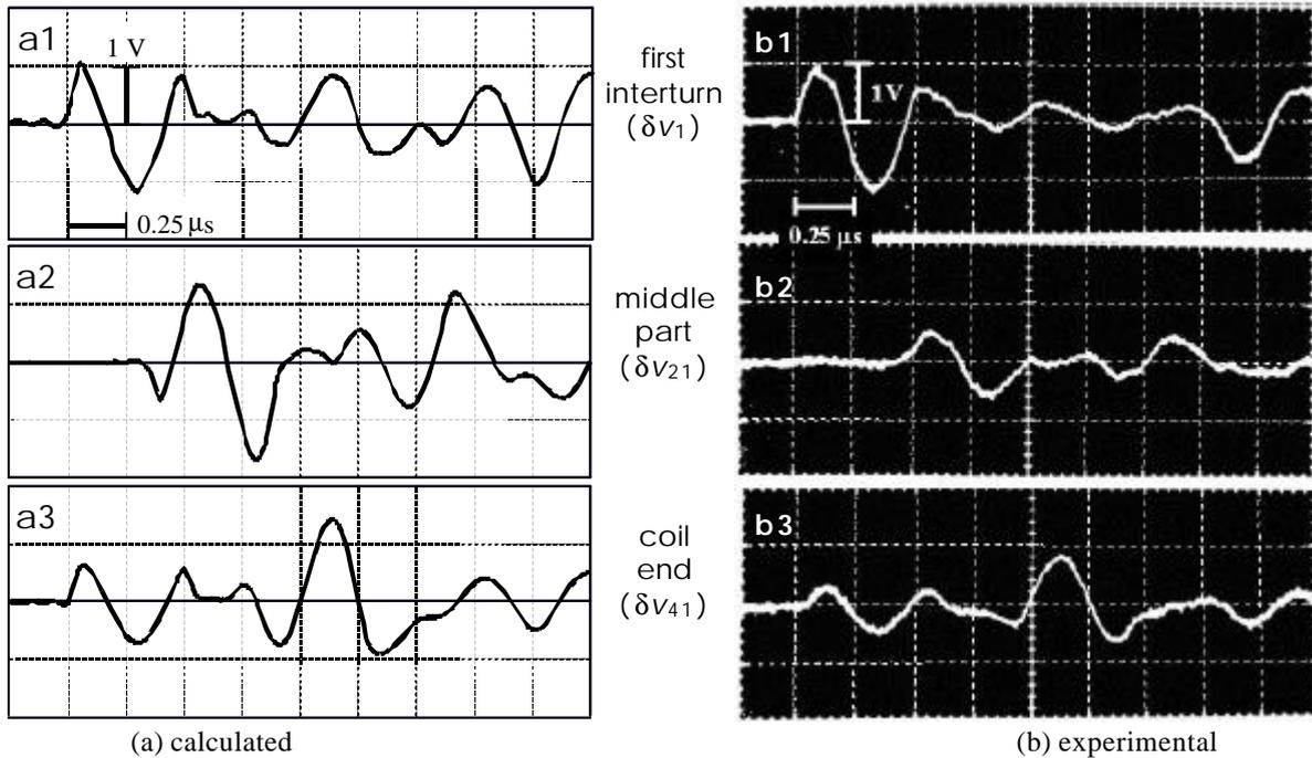
Fig. 10. Interturn voltage waveforms of 2-coil model at application of sinusoidal pulse.
