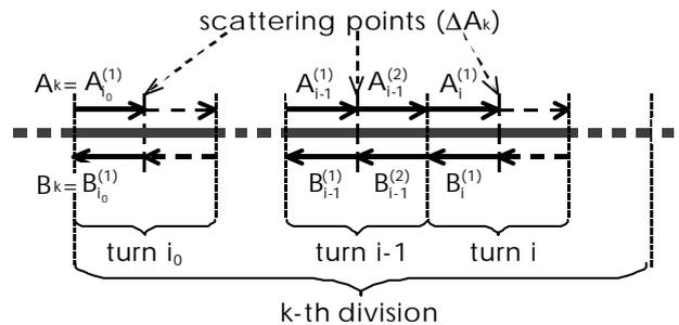
Fig. 3. Travelling waves in a multiple-turn division.
