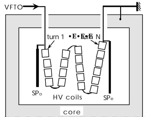
Fig. 1. Shell-form transformer winding.
