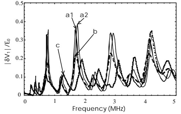
Fig. 7. Frequency characteristics of first interturn voltage for 2-coil model
