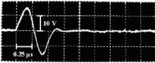
Fig. 9 Sinusoidal pulse used as input voltage in the experiment.
