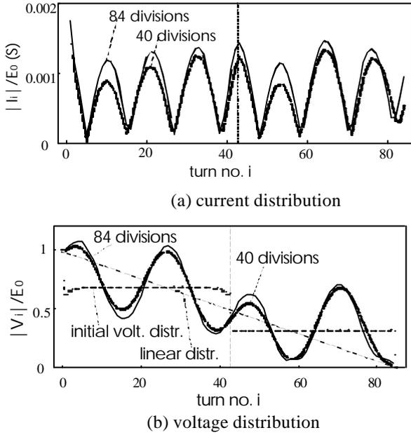
Fig. 6. Current and voltage distributions in 2-coil model at 1.5 MHz.
