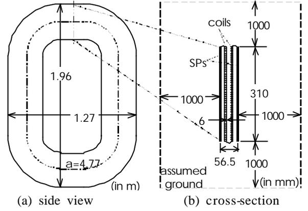
Fig. 4. Configuration of 2-coil model
